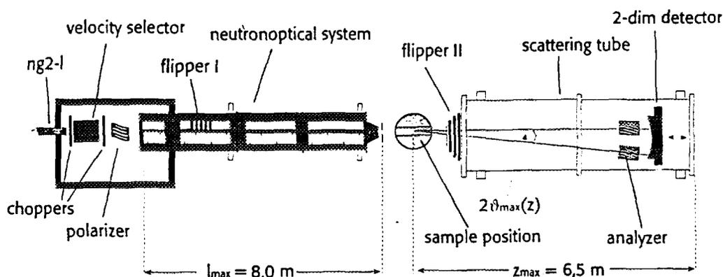
Fig.3 Schematics of the polarized neutron reflectometer PNR at Geestacht presently under construction.
