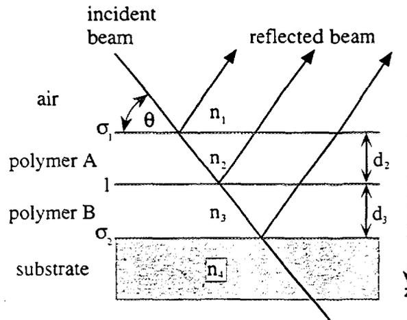
*Fig.1 Schematics of a neutron reflectivity experiment from two polymer films deposited on a substrate. Parameters indicated are film thicknesses  $d_i$ , indices of refraction  $n_i$ , interface widths  $\sigma_i$  and the angles of the incident and transmitted beam  $\theta_i$ , respectively.*
