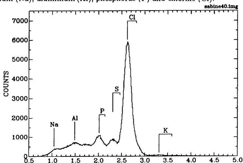
Fig.1 X-ray energy spectrum collected from the sample.
