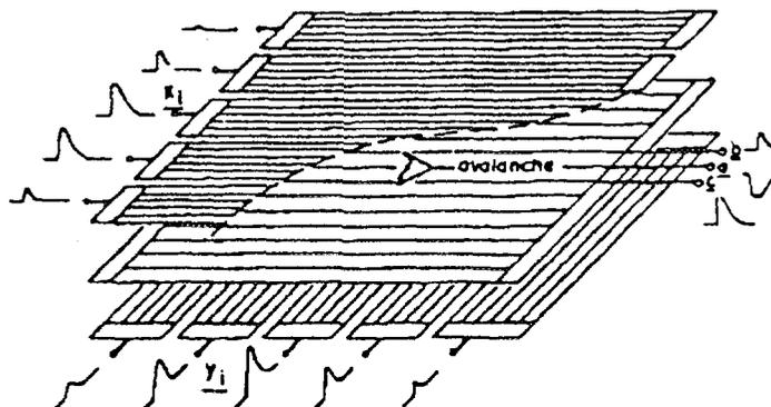
Figure 13 Principle of the center-of-gravity localization method by read-out of the induced charges on cathode planes (43).
