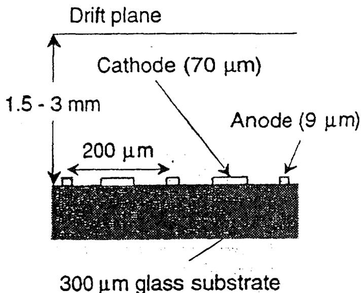
Fig. 9. Electrode configuration of a MSGC
