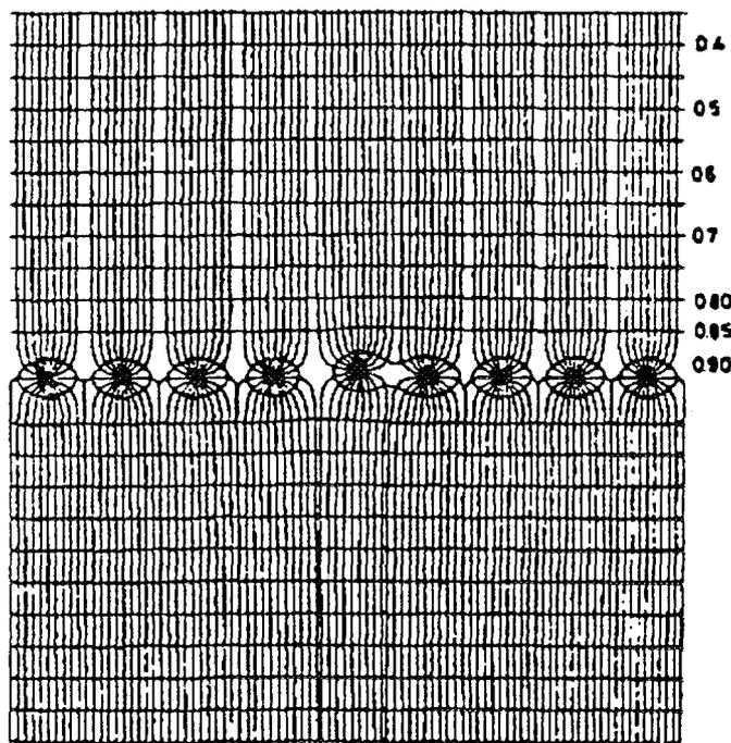
Fig. 6. Electric field equipotentials and field lines in a MWPC. The effect on the field of a small displacement of a wire is also shown.
