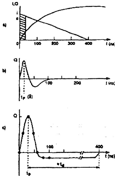
Fig. 21. Signals in a LAr calorimeter: (a) current and induced charge, (b) fast bipolar shaping and (c) the observed signal which is a convolution of (a) and (b) <sup>21</sup>
