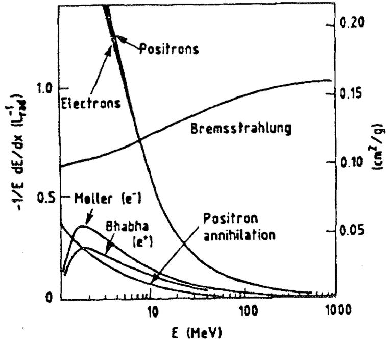
Fig. 15. Fractional energy loss per radiation length (left ordinate) and per  $\text{g}/\text{cm}^2$  (right ordinate) in lead as a function of  $e^\pm$  energy <sup>1</sup>
