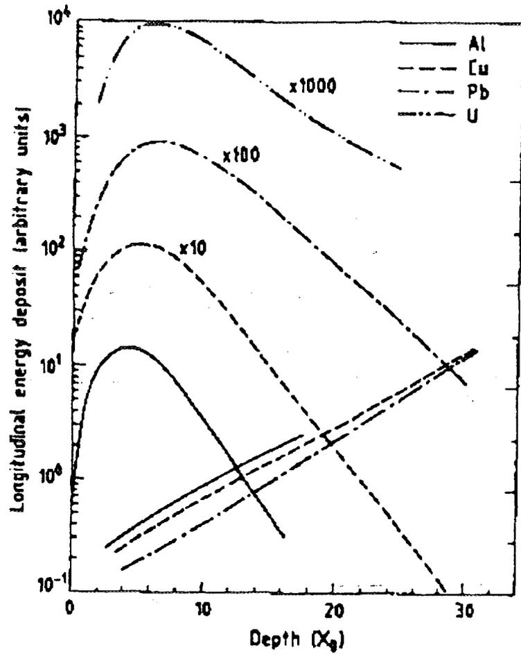
Fig. 17. Longitudinal shower development of 6 GeV electrons in Al, Cu, Pb, U, showing the scaling with the radiation length  $X_0$ .
