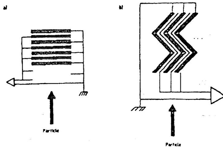
Fig. 19. Sketch of (a) the conventional and (b) the accordion absorber read-out arrangement in a LAr sampling calorimeter
