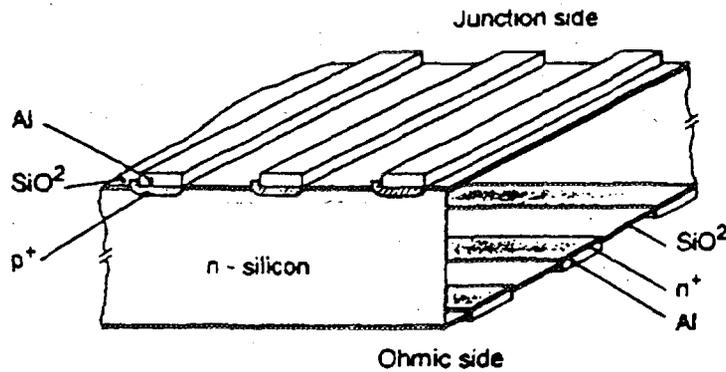
Fig. 12. Sketch of a double sided microstrip detector
