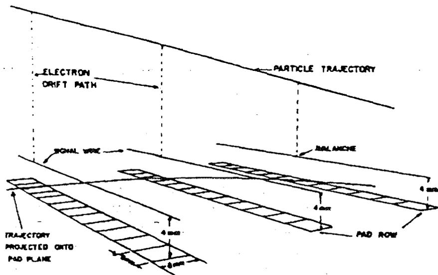
Fig. 8. Sketch of a Time Projection Chamber and of its operating principle
