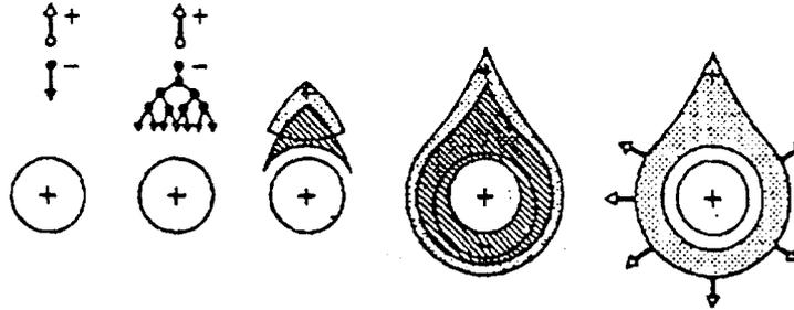
Fig. 3. Pictorial view of charge drift and multiplication in a cylindrical geometry. Time moves from left to right, dark shadow indicates electron cloud, light dark indicates ion cloud <sup>3</sup>
