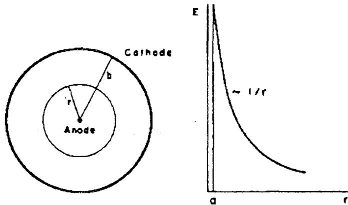
Fig. 2. Geometry of a cylindrical counter and electric field radial dependence
