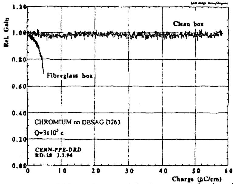
Fig. 11. Gain variation in a MSGC as a function of the charge accumulated on the electrode. Two different gas system have been used: a clean gas system made of inox (upper curve) and a gas system containing plastic and fibreglass (lower curve)
