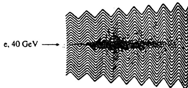
Fig. 20. Simulation of a shower inside the accordion geometry
