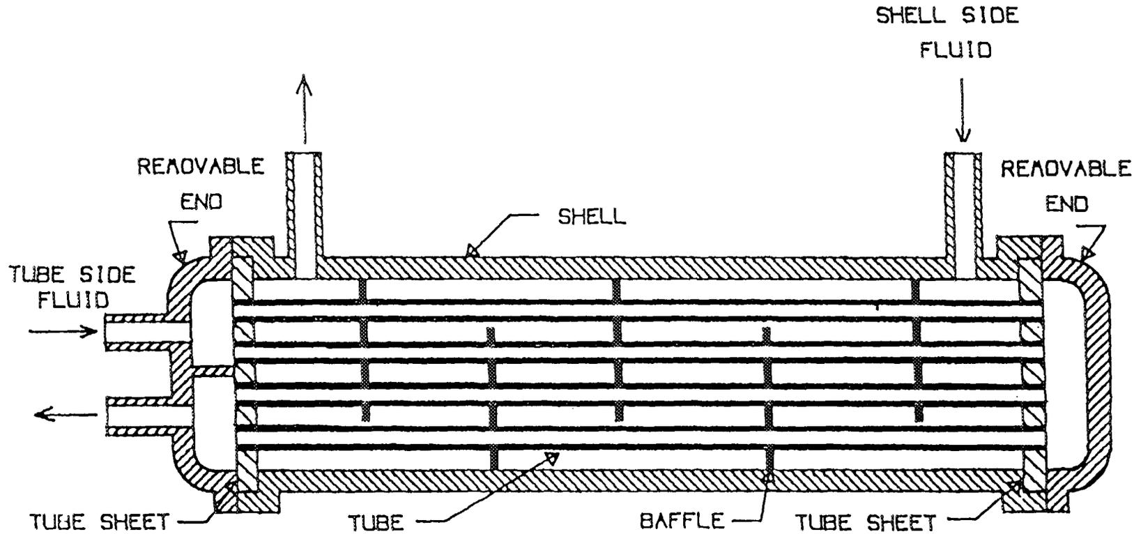
SHELL AND TUBE HEAT EXCHANGER
