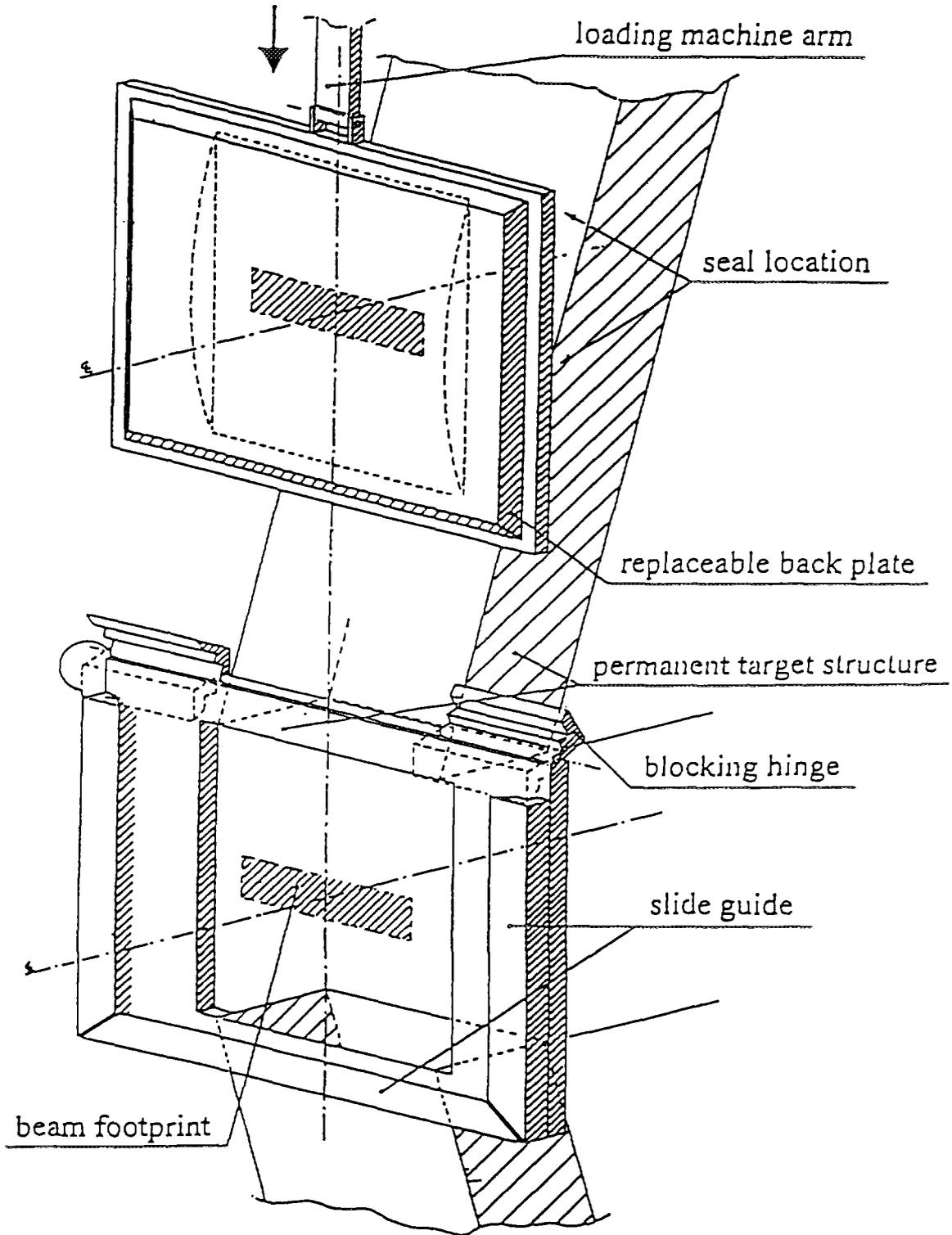
Fig. A2.5-1. The schematic of the bayonet concept.
