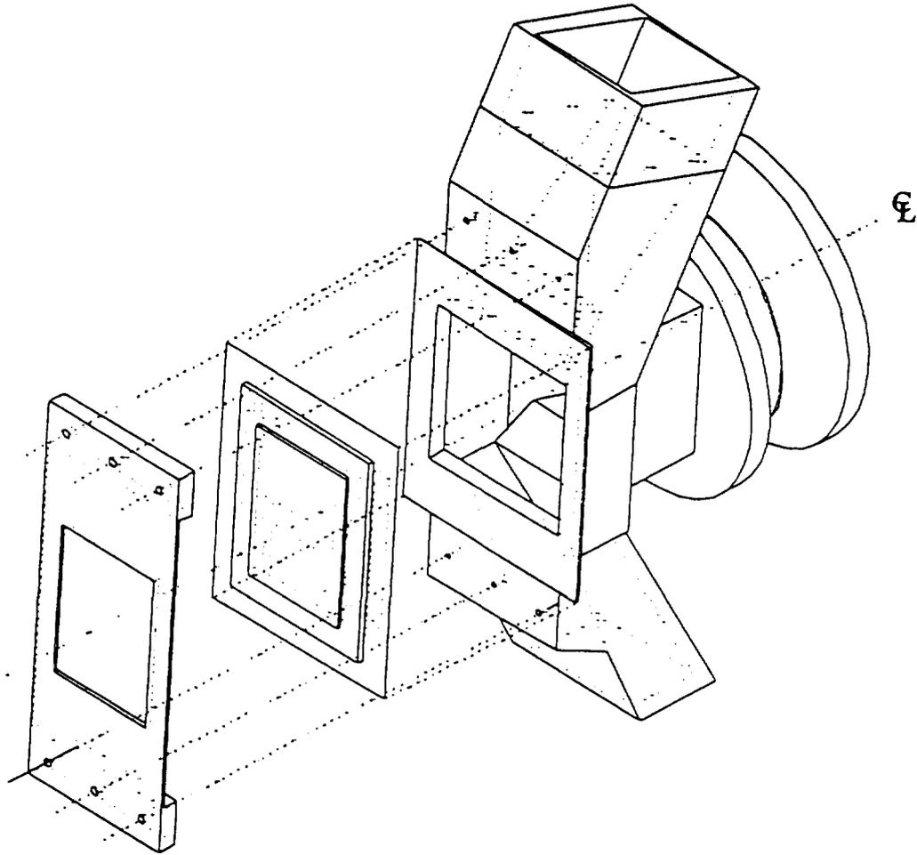
Fig. A2.5-3a. Replaceable backwall attachment scheme.
