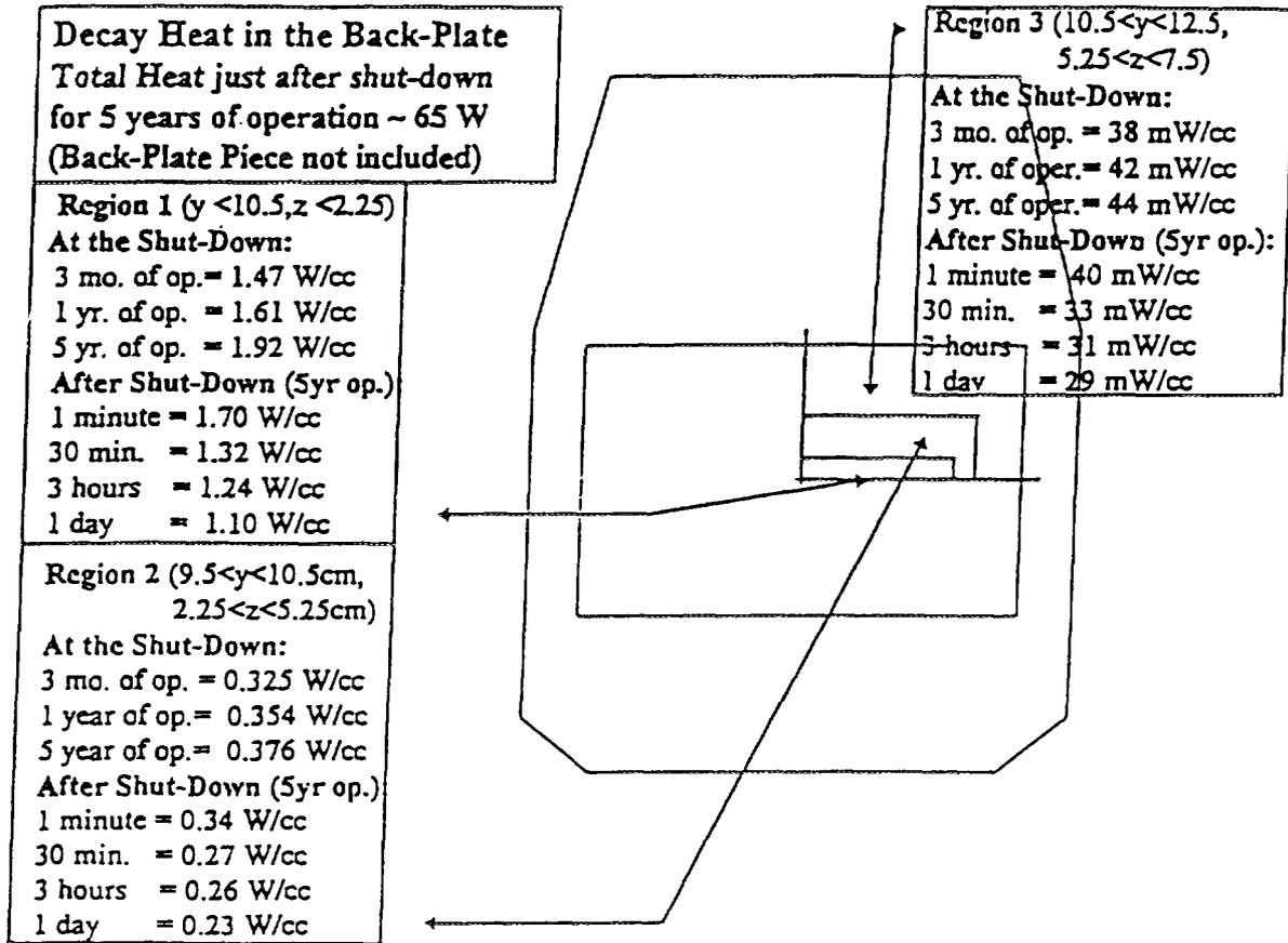
Fig. A2.5-5. Decay heat in the back-plate.
