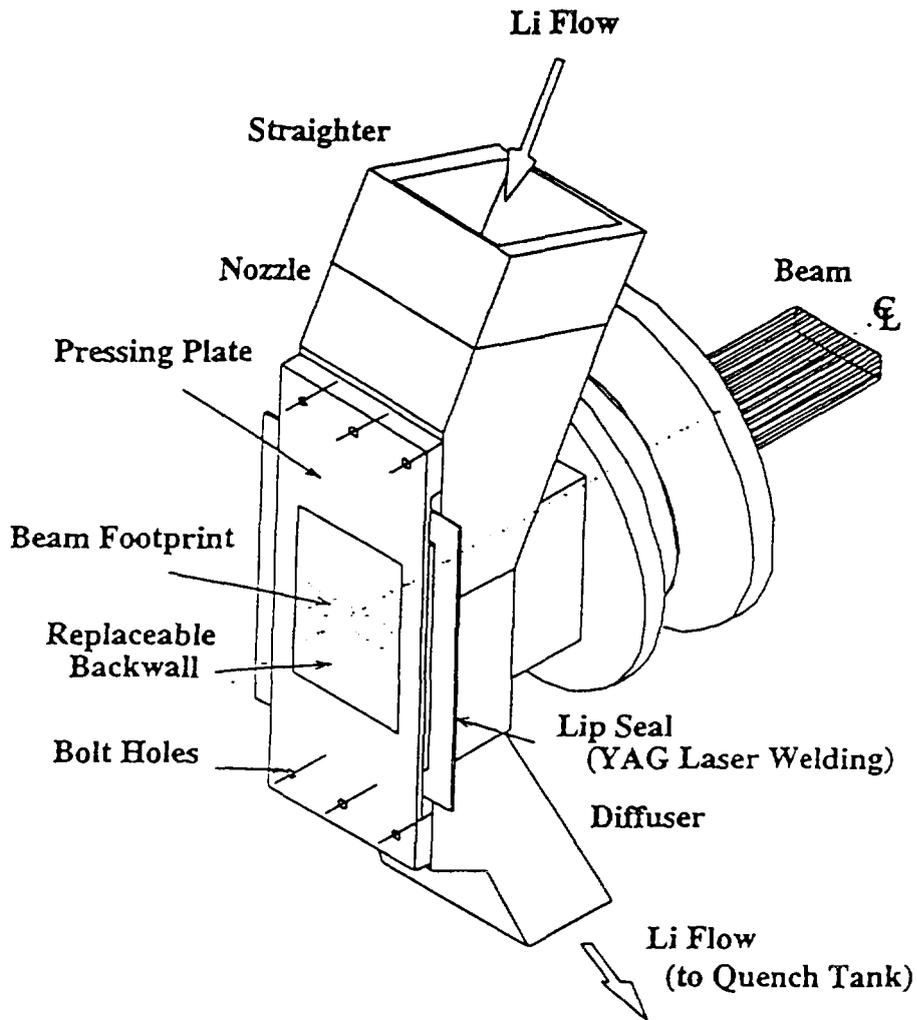
Fig. A2.5-3b. Replaceable backwall attachment scheme.
