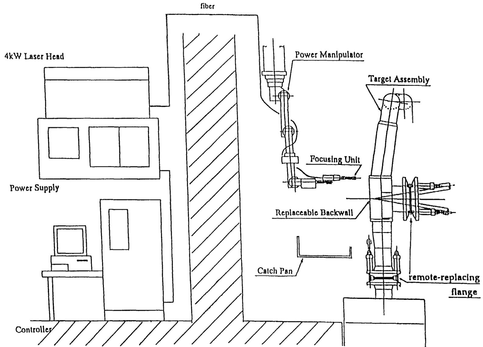
Fig. A2.5-2. Schematic of the YAG laser processing system.
