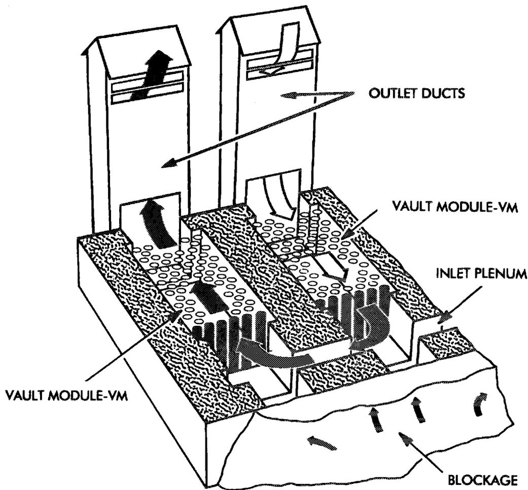
Figure 8 Cooling regime as result of duct blockage
