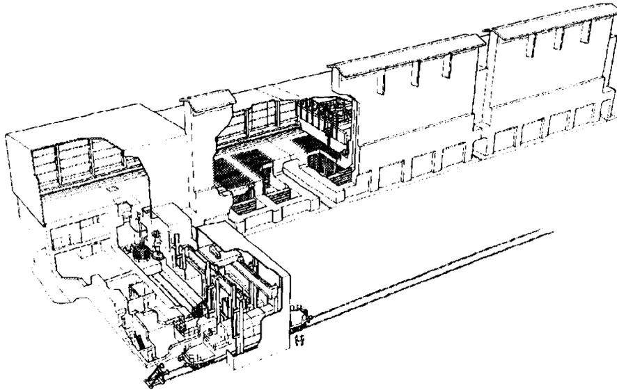
Figure 3 Paks NPP - Modular vault dry store
