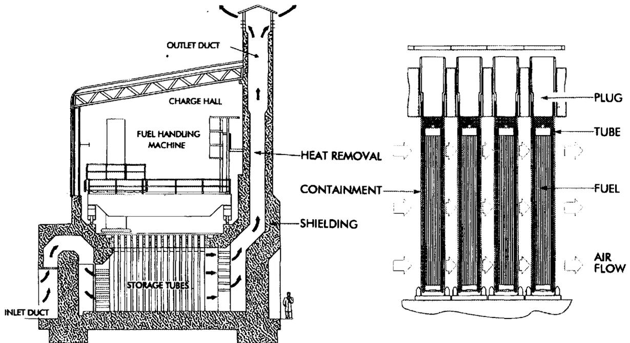
Figure 1 Modular vault dry store - cooling system
