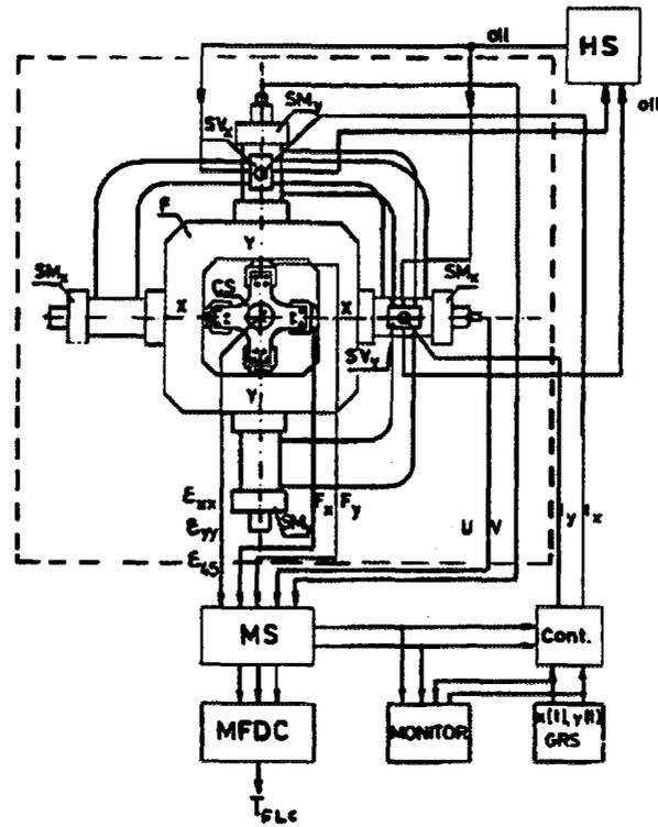
Figure 7. Experimental fatigue testing machine
