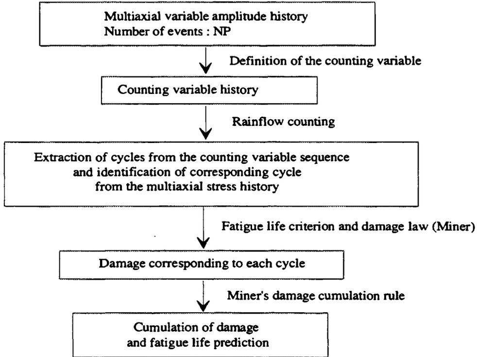
Flow chart of the proposed stress-based fatigue life prediction method
