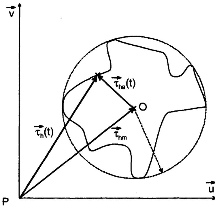
Figure 4. Definition of the shear stress amplitude
