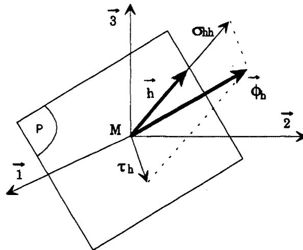
Figure 2. Definition of the stress vector acting on a physical plane.
