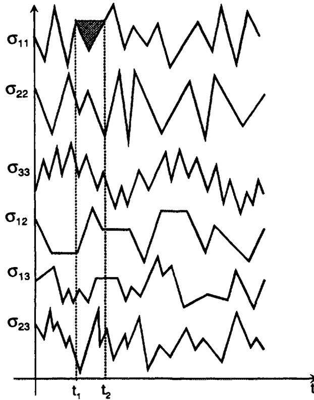
Figure 1. Problem of cycles counting for multiaxial variable amplitude stress states
