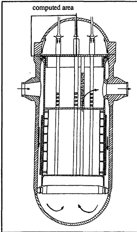
Figure 1 - General view of a pressurised water reactor
