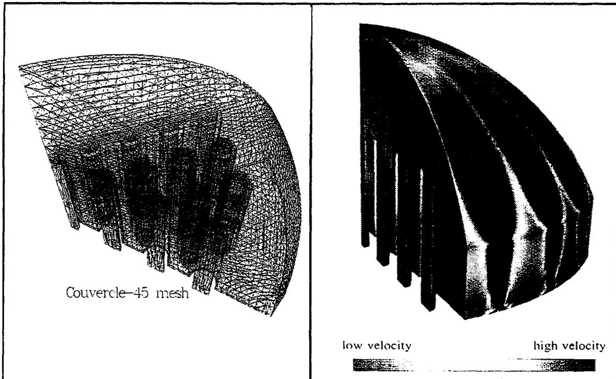
Figure 3 - Finite element mesh of a 45° sector of a reactor upper head
