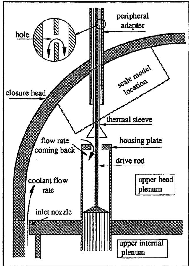
Figure 2 - Global view of the upper head geometry with one adapter
