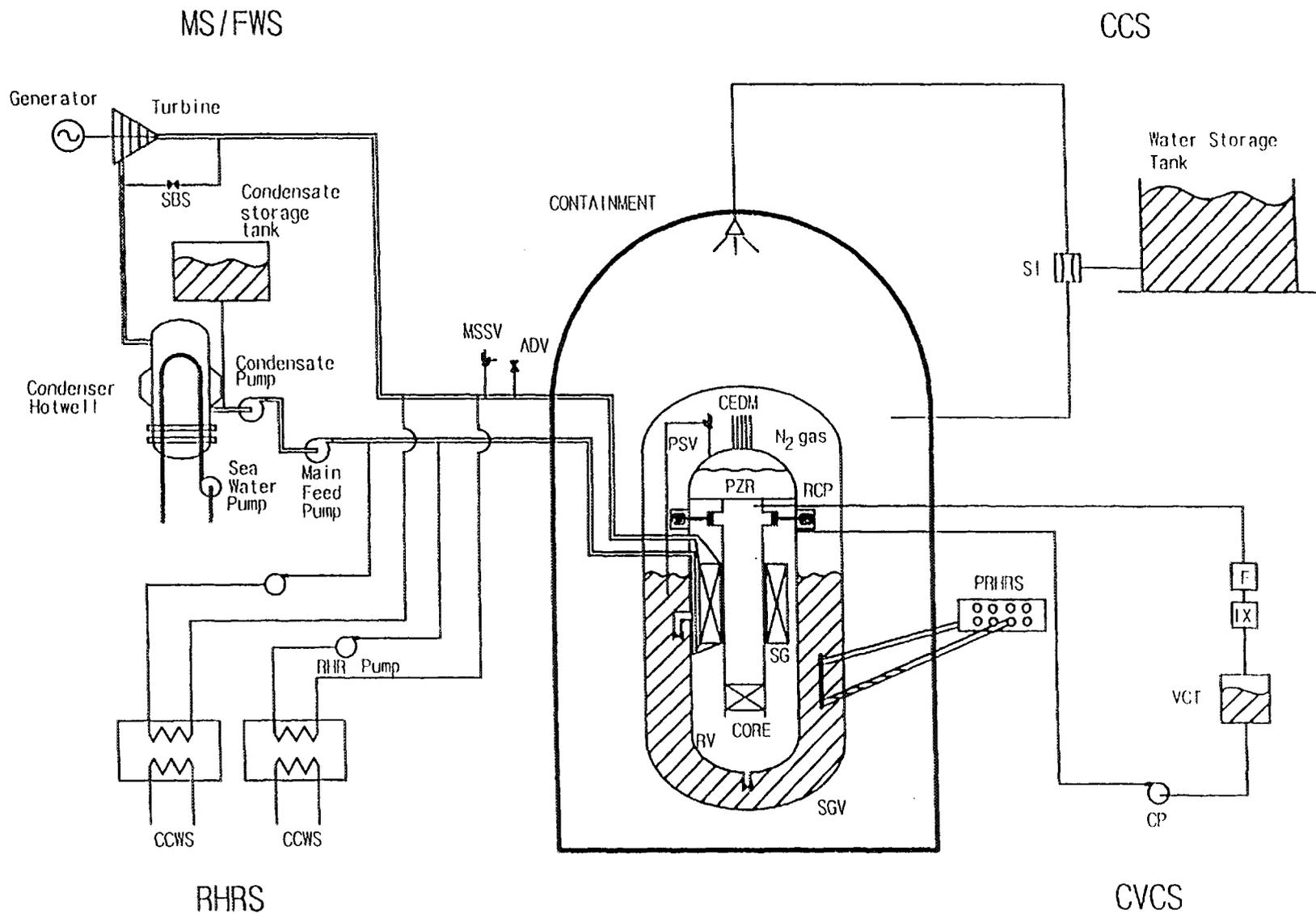
FIG. 3. Schematic diagram of advanced integral reactor systems.
