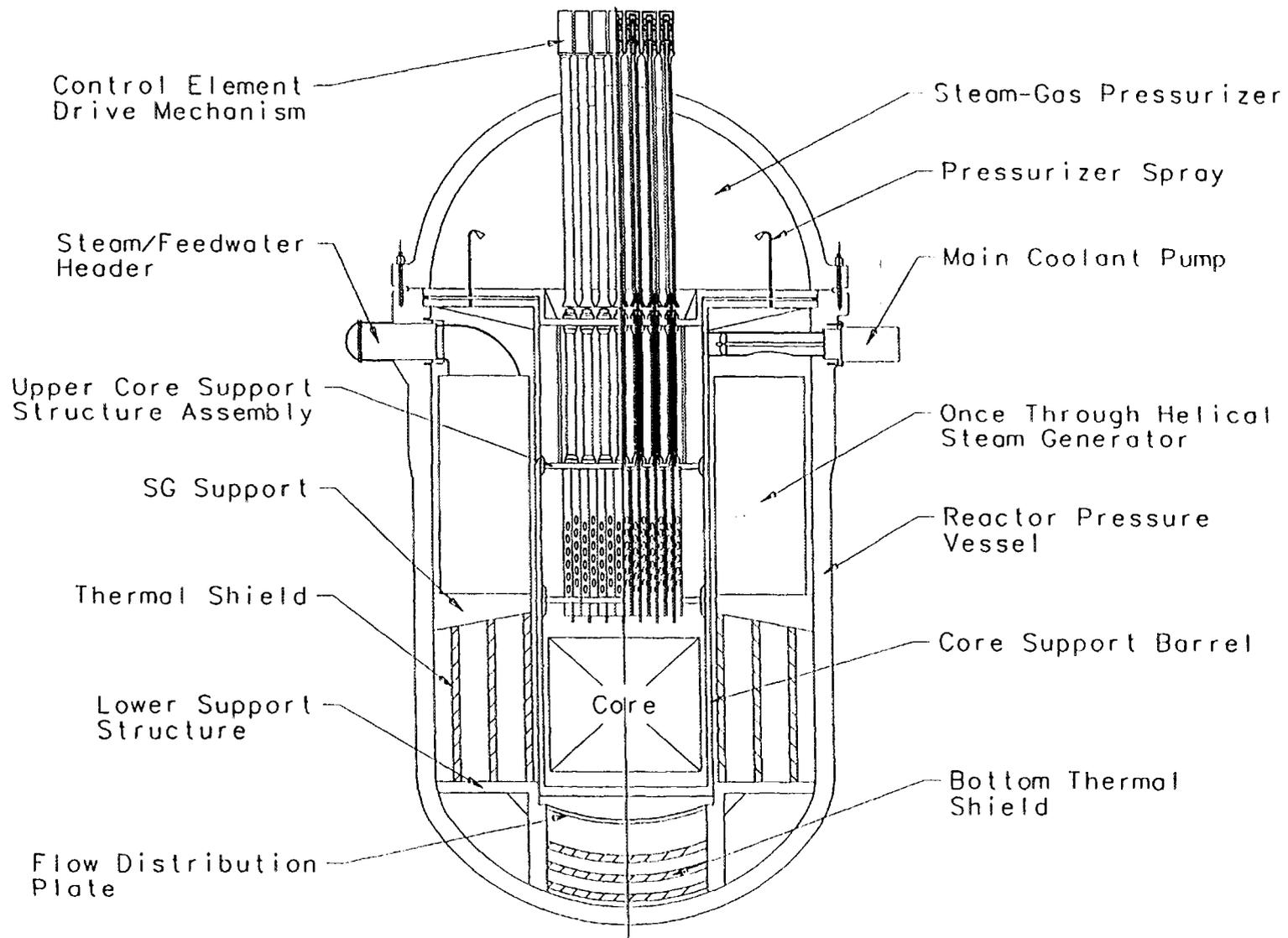
FIG. 2. General arrangement of primary components and reactor internals.
