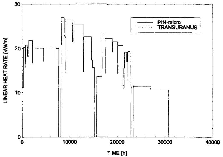
**Figure 1 Local linear heat rate, FA 1**
