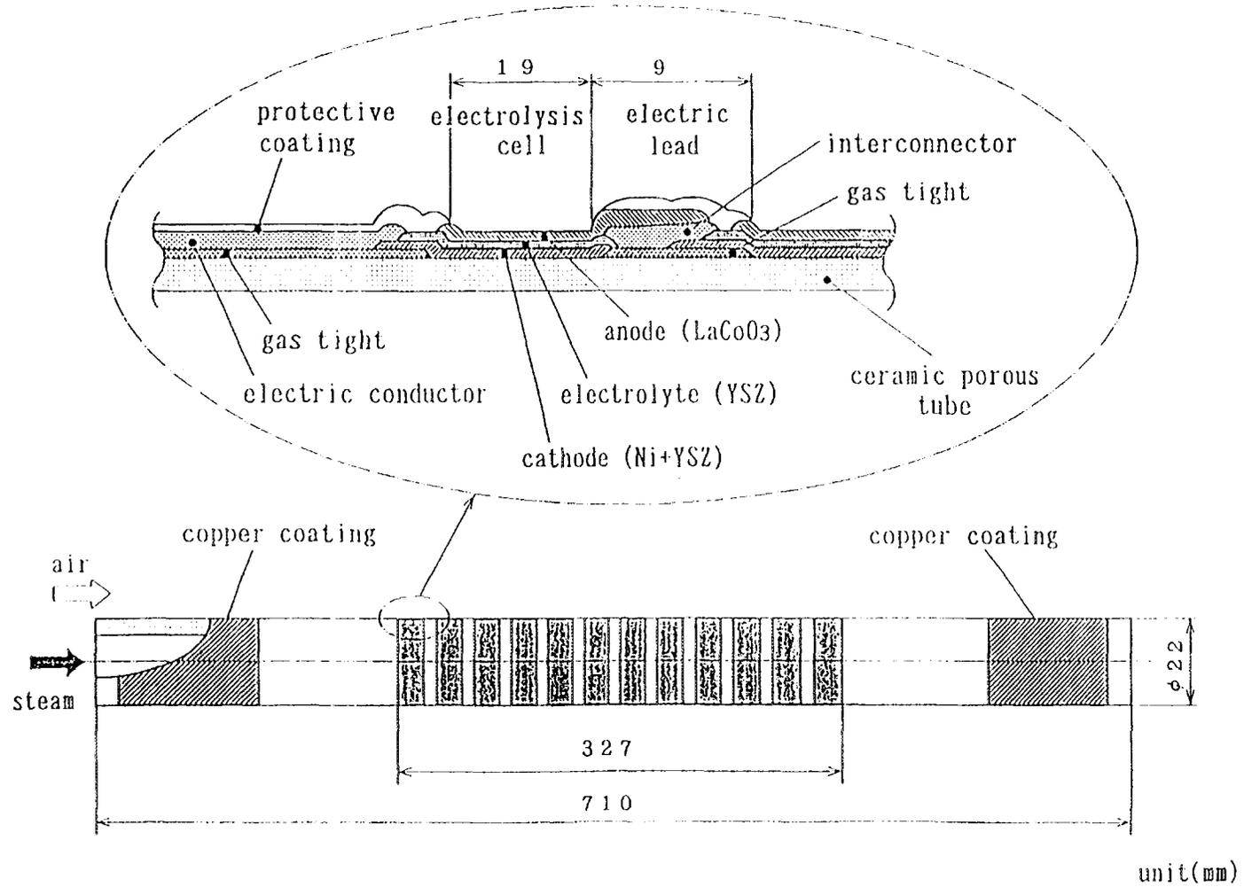
Fig. 2 Electrolysis tube with 12 cells [6]
