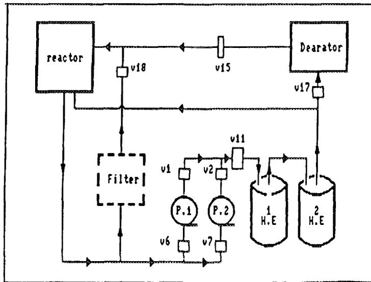
Fig. 6 Block Diagram of The Reactor Cooling Circuit
