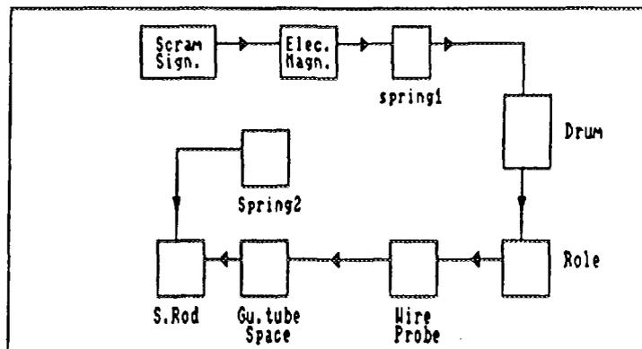
Fig. 7 Block Diagram of The Safety Rod Mechanism
