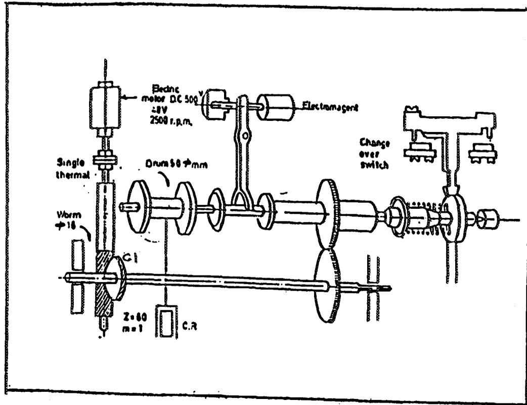
Fig. 3 Safety Rod Mechanism
