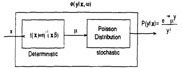
Figure 3: Poissonian Model of a  $\gamma$  spectrum channel.
