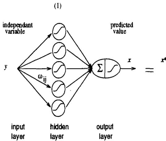
Figure 4: MLP 3-5-1 with nonlinear threshold.
