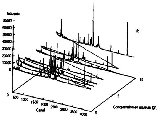
Figure 2: 3D-Representation of the  $UO_2$  spectra set.
