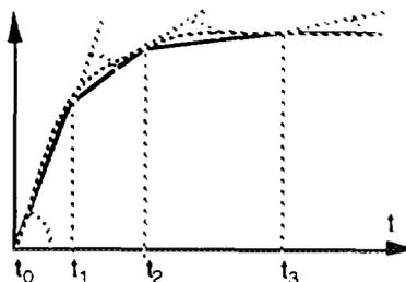
Figure 2 : Response by a first order QTF to a step input
