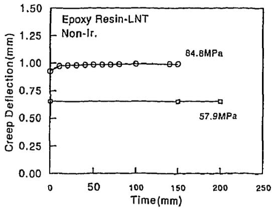
Fig. 2. Creep curves for non-irradiated epoxy-resin at LNT.
