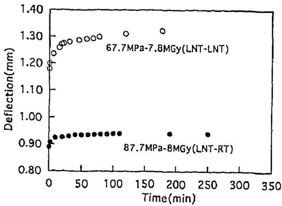
Fig. 4. Comparison of creep curves at LNT for irradiated epoxy resin between with and without raising to RT.
