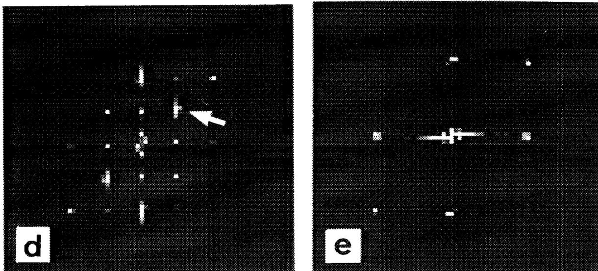
Figure 5: Bright-field (a) and dark-field (b) images showing both orthorhombic particles (A and B) and tetragonal particles (C, D, E and F). (c) High resolution micrograph showing images of particle B and C. (d) Fourier transform of digitized selected image area from orthorhombic particle (B). (e) Fourier transform of digitized selected image area from tetragonal particle (C).
