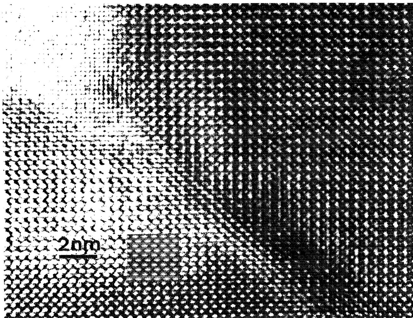
Figure 2: High resolution micrograph showing images of two adjacent orthorhombic particles in  $[001]_o$  orientation (inset is a calculated image).
