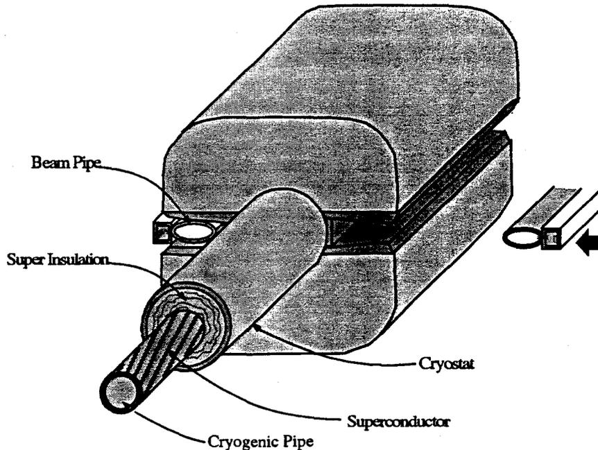
Fig. 1: Double-C twin bore transmission line magnet
