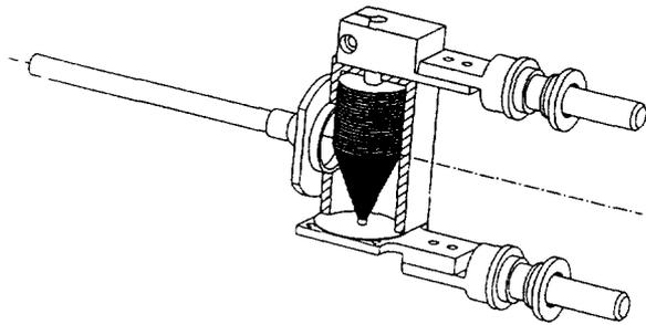
Fig. 4 : Structure of the conical target
