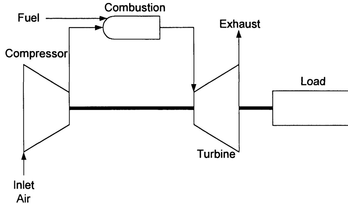
**Fig. 3 Simple-cycle, single-shaft gas turbine**
