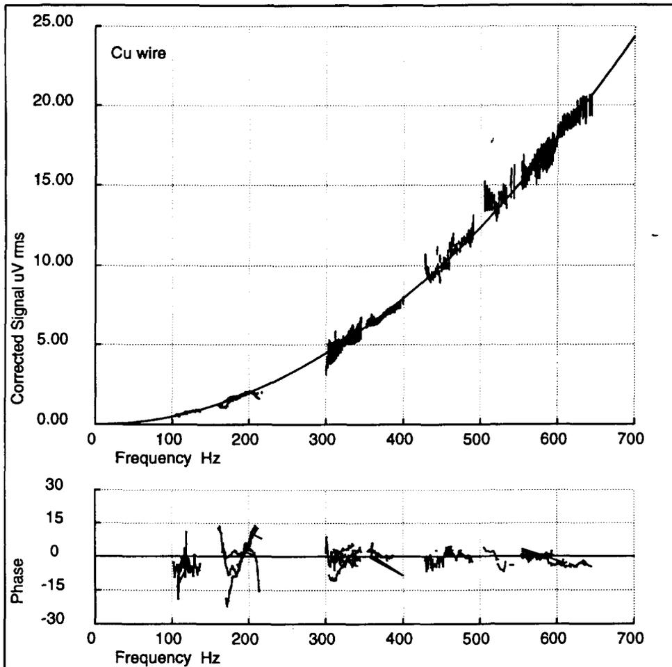
FIG. 4. Summary of Copper data corrected for separately measured rotation amplitude and coil areas plotted against frequency to show the expected quadratic behaviour. The solid lines represent the theoretical predictions. Similar results were obtained for Aluminium.
