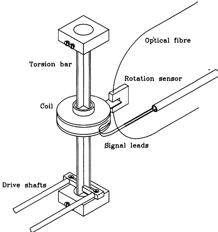
FIG. 1. Sketch of the test coil and torsion bar. Note the cross-shaped cross-section of the bar, chosen to separate flexural and torsional vibration modes by making the bar much stiffer in bending than in torsion. Excitation was provided by two push-rods vibrating in anti-phase. Note shown are rigid frame and massive support structure on which the assembly was mounted, nor the vibration-isolated three-axis set of Helmholtz coils to eliminate the constant geomagnetic field.
