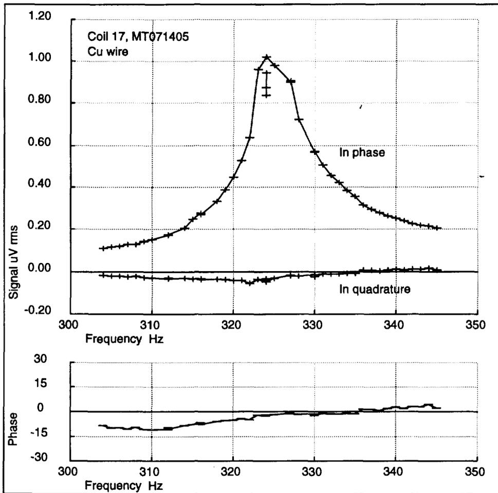
FIG. 2. Coil voltage amplitude and phase data from a typical experimental run. The solid line connects theoretically predicted values.
