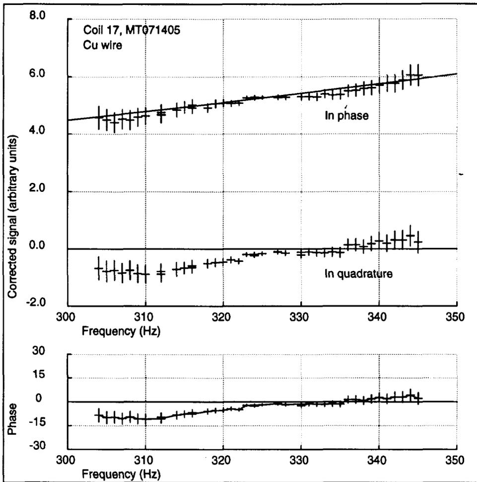
FIG. 3. The same data as the experimental run of the previous figure adjusted for rotation amplitude to a common reference value using the rotation transducer measurements. The solid line shows the theoretically predicted signal parabolic with frequency.
