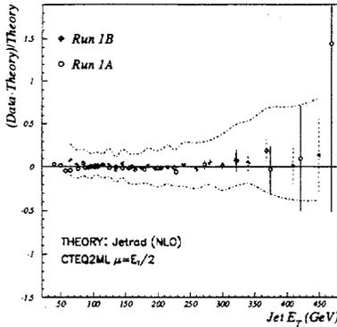
Figure 1: A comparison of the central,  $|\eta| \leq 0.5$ , inclusive cross section to a NLO QCD calculation with CTEQ2ML evaluated at  $\mu = E_T/2$  of the leading jet. The points only include statistical errors. The band represents the total systematic error except the luminosity uncertainty. The solid (open) symbols are for the 1994–1995 (1992–1993) data.
