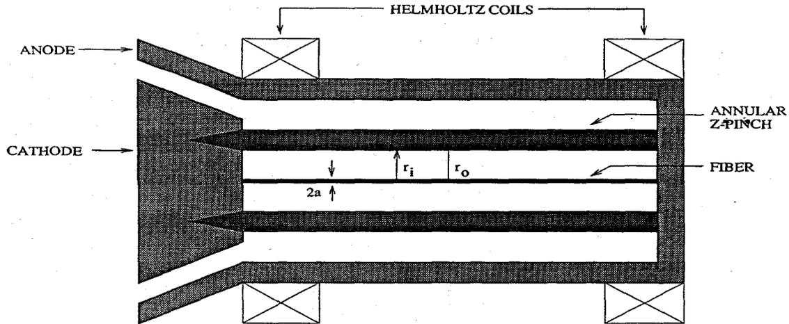
Figure 1. Staged Z-Pinch.
