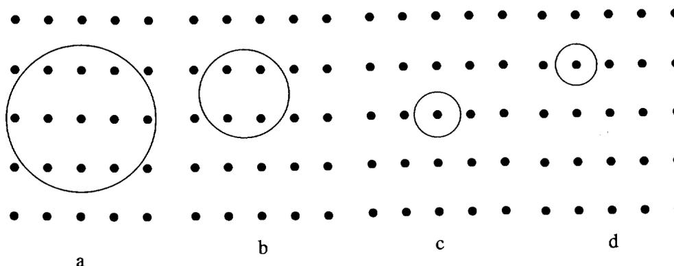
Figure 3: Illustrating the beams included in the objective aperture for (a) many-beam bright-field, many-beam dark-field, single beam bright-field (c) and single-beam dark-field.
