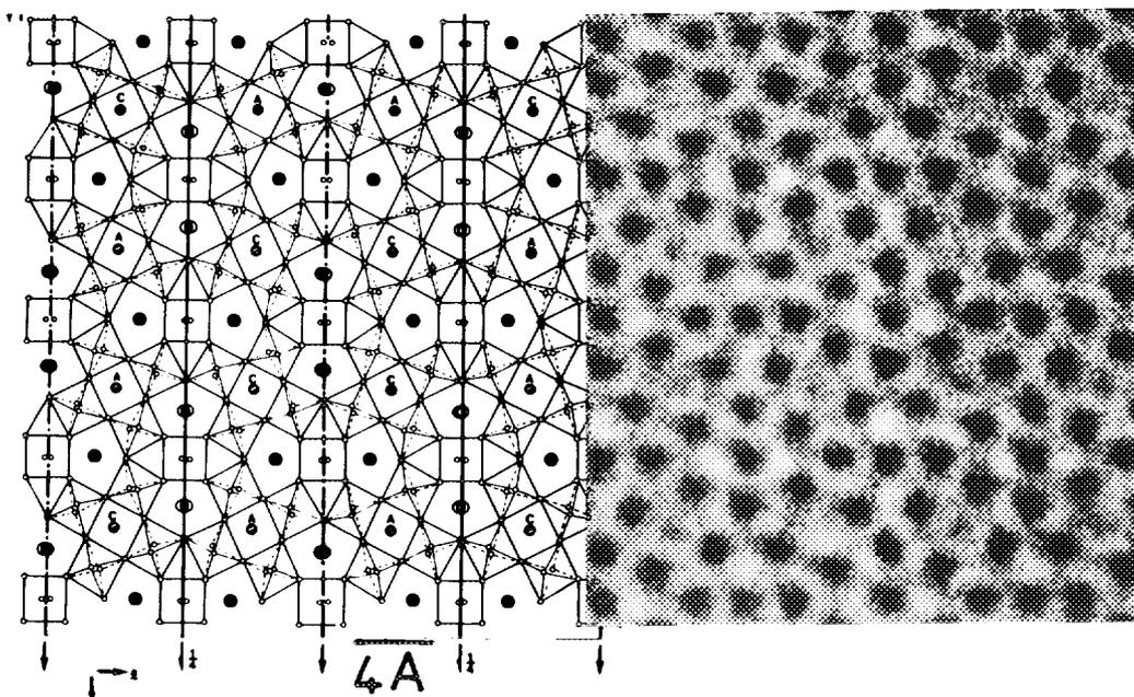
Figure 2: HRTEM image of barium sodium niobate; note correspondance between black spots and the cation positions,
