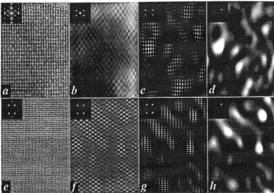
Figure 5: (a) Digitized image of experimental image of PMN; (e) computer simulated image of PMN; (c-h) show details of the image reconstructions referred to in detail in the text; insets are power spectra.
