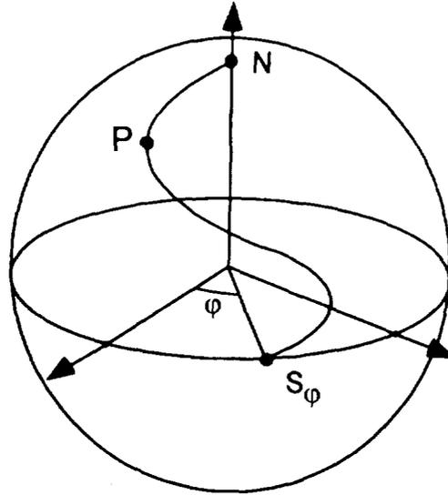
FIG. 1. Representation of the proximity effect: The point  $P$  follows a trajectory going from a normal reservoir (N) to a superconducting reservoir with phase  $\varphi$  ( $S_\varphi$ ).
