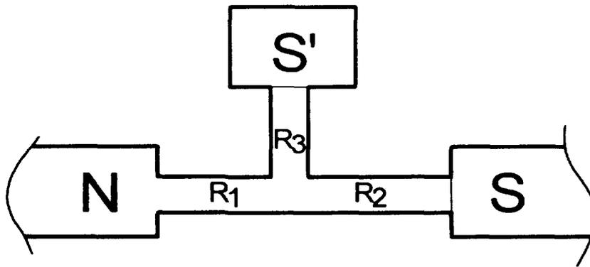
FIG. 3. Example of diffusive NS structure in which the resistance is strongly modified by the proximity effect. The resistance  $R$  between the N and S reservoirs  $R = R_1 + (R_2^{-1} + R_3^{-1})^{-1}$  depends on the resistance  $R_3$  of the dangling arm.
