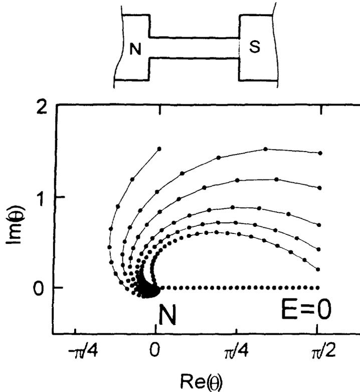
FIG. 5. Variations of the proximity angle  $\theta$  along a N wire of length  $L = 5L_{\Delta}$  connected at its ends to a normal and to a superconducting reservoir. The distance between successive points is  $0.2L_{\Delta}$ . The energies are  $E/\Delta = 0, 0.2, 0.4, 0.6, 0.8, 0.9, 1.1$ .
