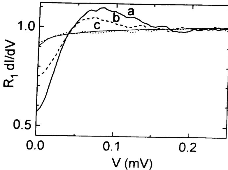
FIG. 8. Differential conductance as a function of the voltage  $V$  measured at 30 mK and in a magnetic field  $H = 0$  (curve a), 0.06 T (curve b), and 0.1 T (curve c). The thin solid line is a fit of curve c using Eq. (14), in which the DOS  $n(x, E)$  was taken constant. It accounts for the influence of single-electron charging effects on the conductance of a tunnel junction between normal electrodes.
