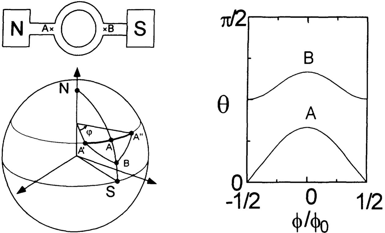
FIG. 4. a) Simple NS circuit with a loop enclosing a flux  $\Phi$  and its representation on the unit sphere. b) Variations of the proximity angle  $\theta$  at points A and B as a function of the flux  $\Phi$ .
