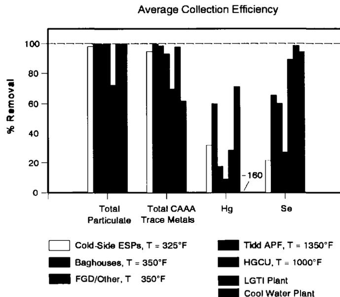
Figure 3. Average collection efficiency for all 11 CAAA trace elements, Hg, and Se for both conventional and advanced control systems.
