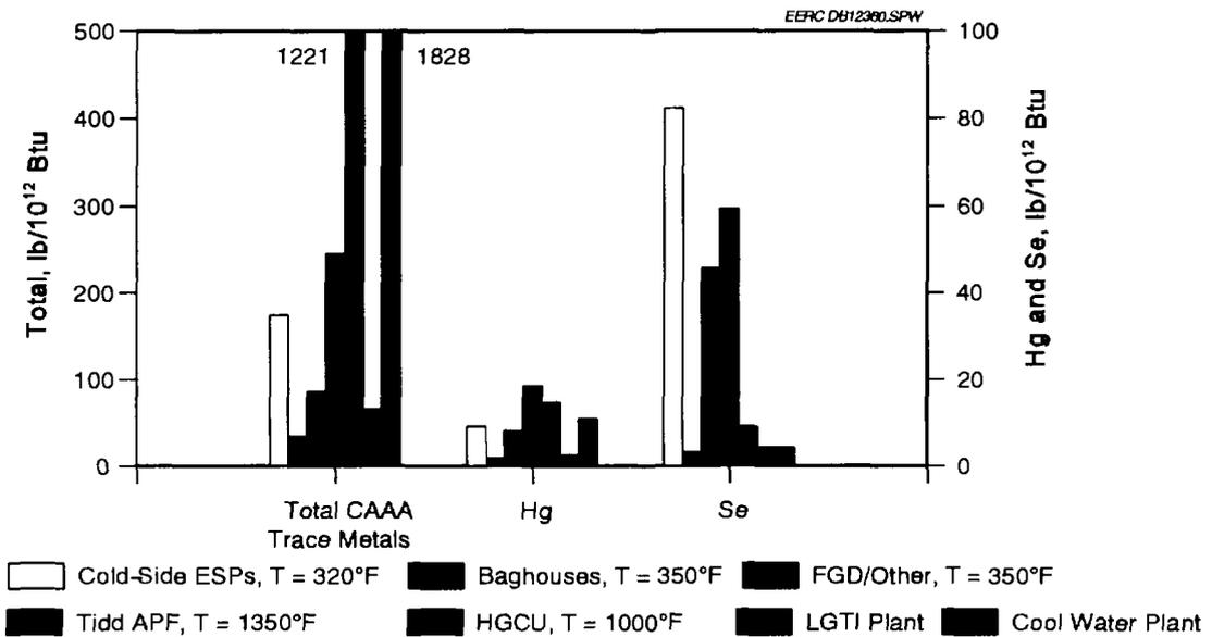
Figure 2a. Summarized emission factors of total CAAA trace elements, Hg, and Se. Note that contamination of Cr and Ni in the Tidd APF outlet samples is suspected. Results from both GE HGCU and Cool Water were subject to sampling error.
