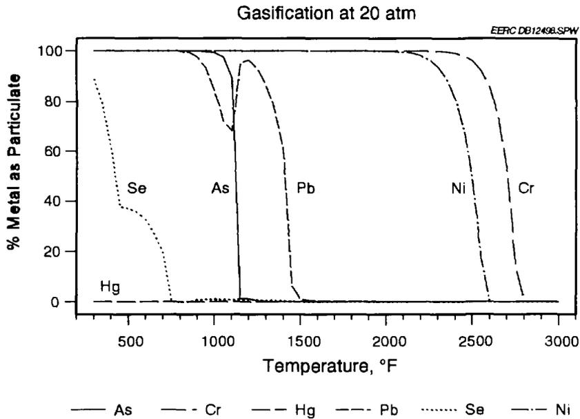
Figure 5. Amount of each element present as particulate as a function of temperature under typical combustion conditions as simulated for an entrained-flow gasifier at 20 atm.
