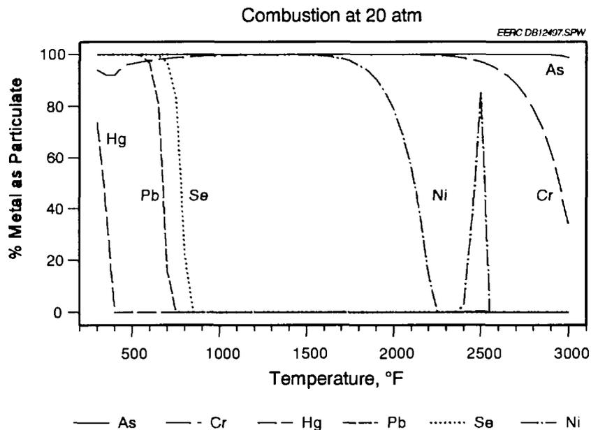
Figure 4. Amount of each element present as particulate as a function of temperature under typical combustion conditions as simulated for the Tidd PFBC system at 20 atm.
