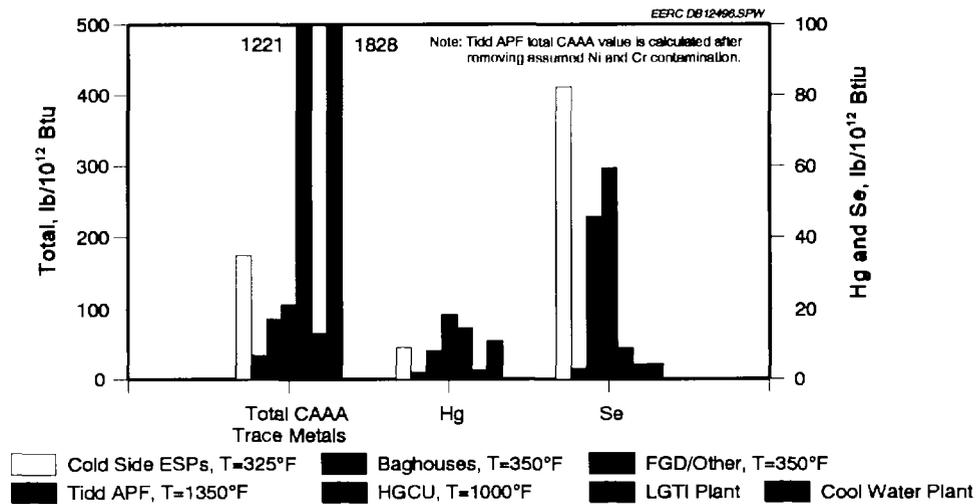
Figure 2b. Summarized emission factors for all 11 CAAA trace elements, Hg, and Se with the Tidd APF total CAAA value corrected for contamination of Cr and Ni.
