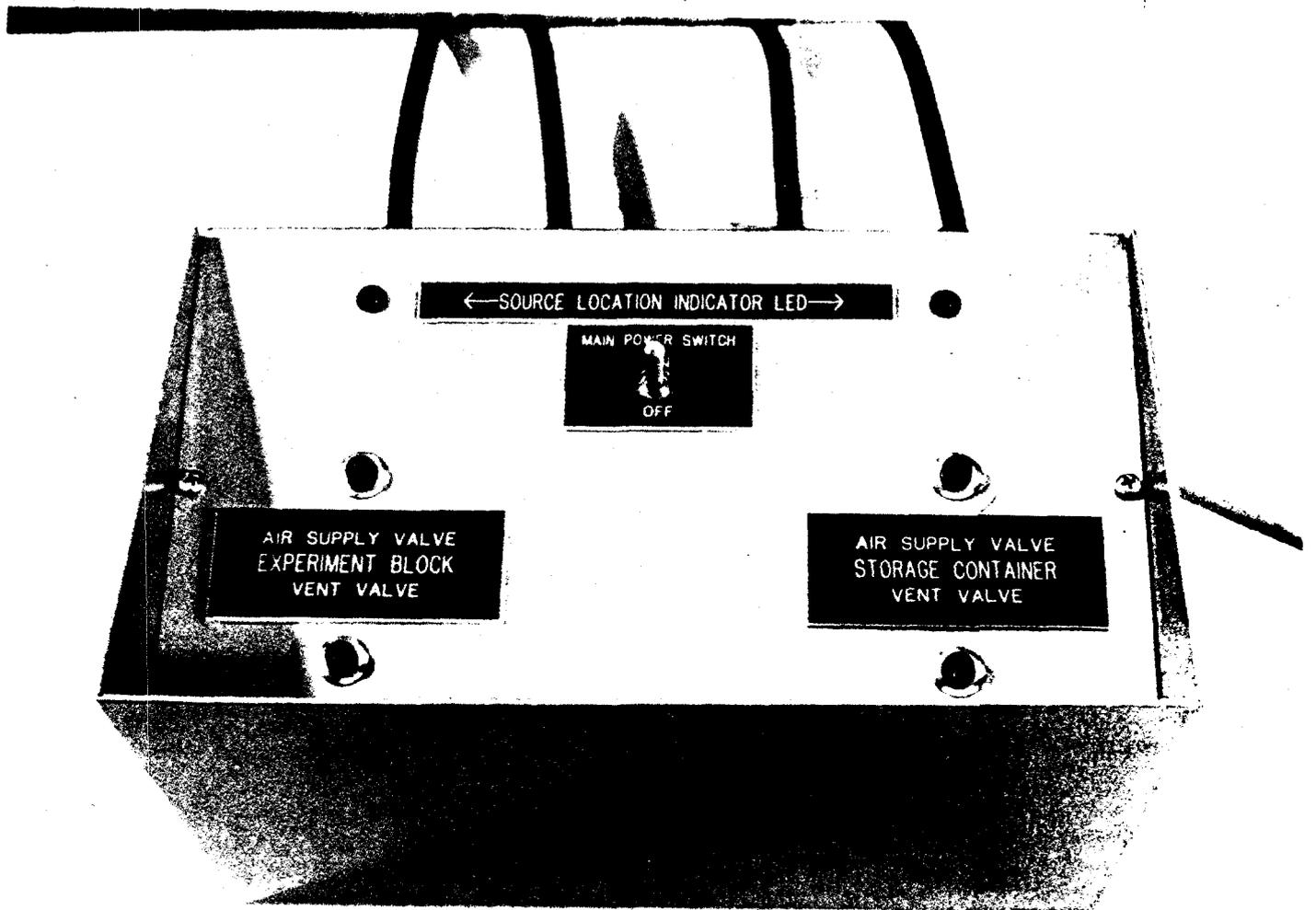
Figure 7. Control box with red indicator LED's at top of box, toggle switch with locking mechanism to prevent accidental activation or deactivation of electrical power, red momentary contact buttons for capsule transfer, black momentary contact buttons to close vent valves.
