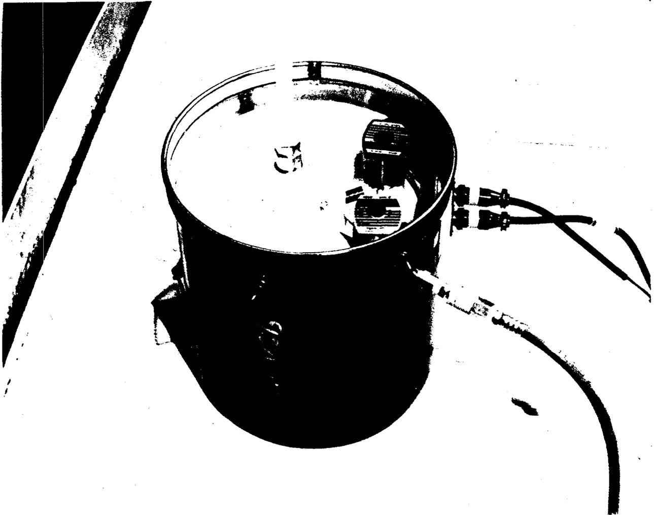
Figure 5. View of the  $^{252}\text{Cf}$  storage drum with the transfer line, electrical connections, and air line attached.
