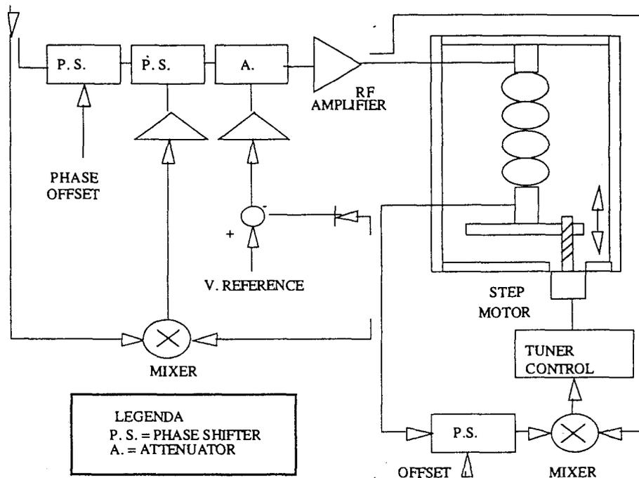
Figure 11 – Stabilization loops : block diagram.
