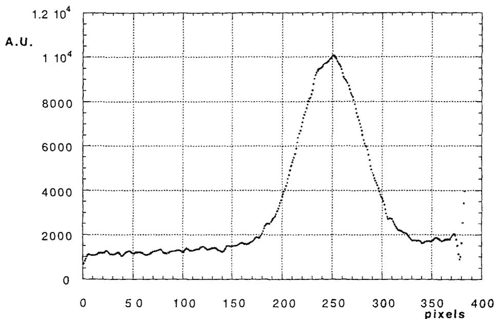
**Figure 20** – Horizontal beam profile from previous image.
