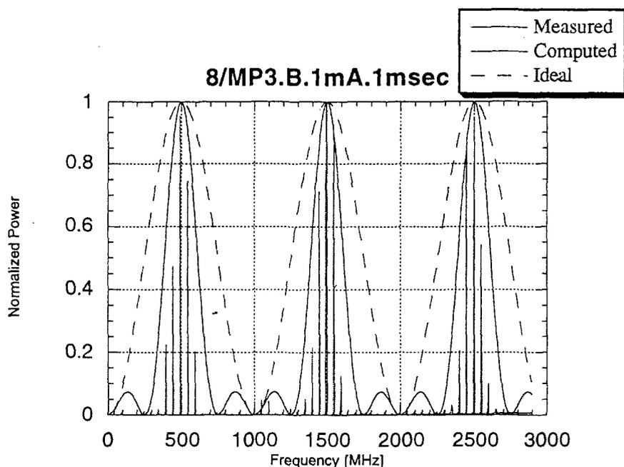
**Figure 7** – Measured spectrum lines, computed and ideal envelopes.
