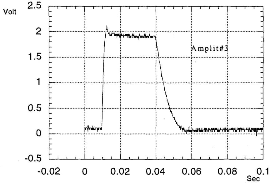
Figure 14 – Typical voltage pulse(1 V=1.5 MV).
