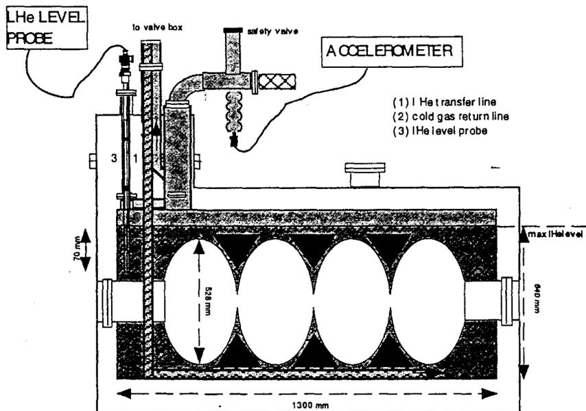
Figure 8 – Sketch of the SC accelerating module.
