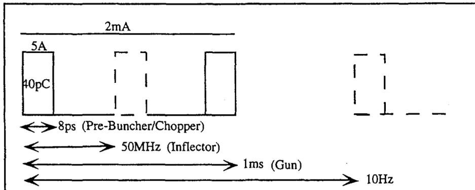
Figure 6 - Beam time structure.
