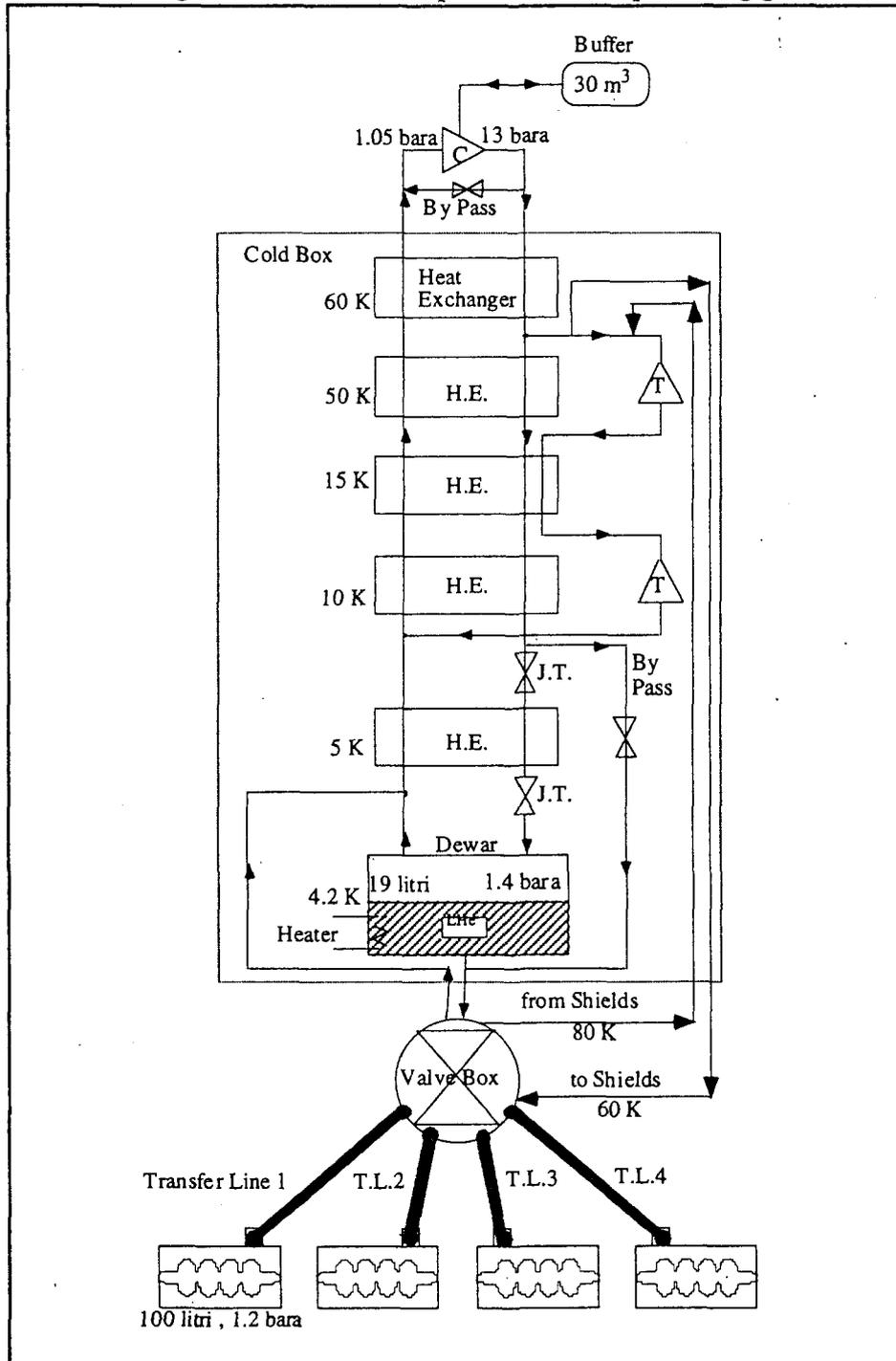
Figure 16 – Sketch of the refrigeration system.
