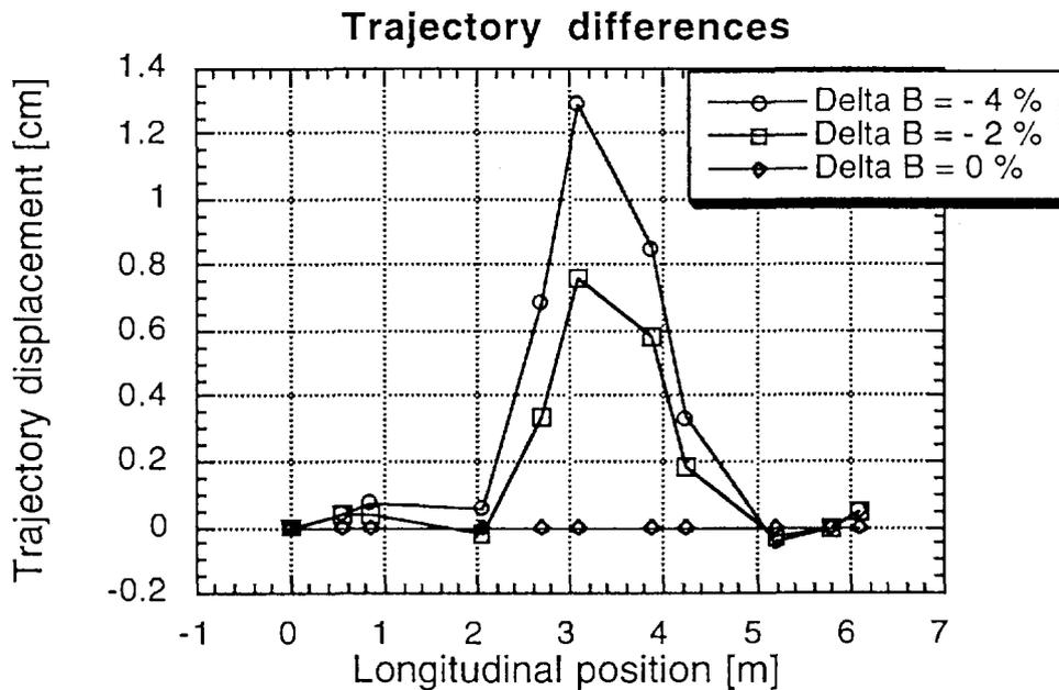
**Figure 21** – BPM measurement of the relative beam displacement in the arc varying the bending field of  $-2\%$  (square points) and  $-4\%$  (dot points).
