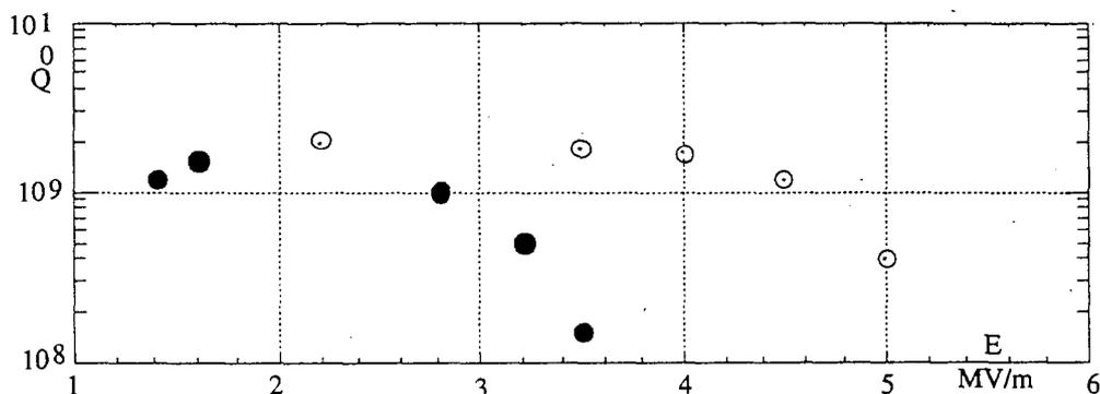
Figure 10 –  $Q_0$  vs. accelerating field  $E$  @ 4.2 K.
