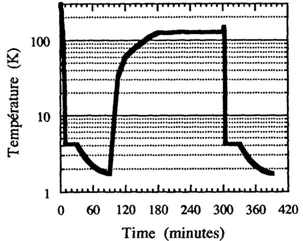
Figure 5. Typical thermal cycle of the dielectric resonator.
