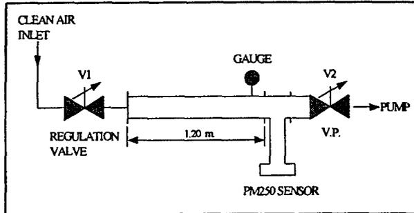
Figure 5.1 : Dust particle transport device
