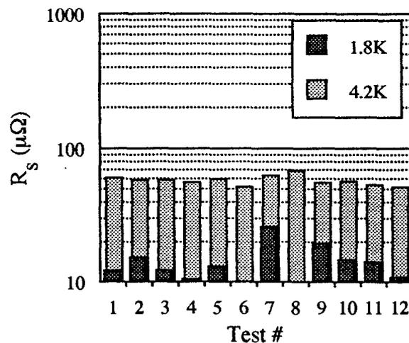
Figure 3. The results of twelve different measurements of surface resistance. The resonator was cooled quickly from room temperature for each test. All measurements were made at 9.52 GHz. Tests 1-5 used chemically polished, high RRR plates. Tests 6-8 used chemically polished, low RRR plates. Tests 9-12 used electropolished, high RRR plates.  $R_s$  at 1.8K was not measured in tests 6 and 8.
