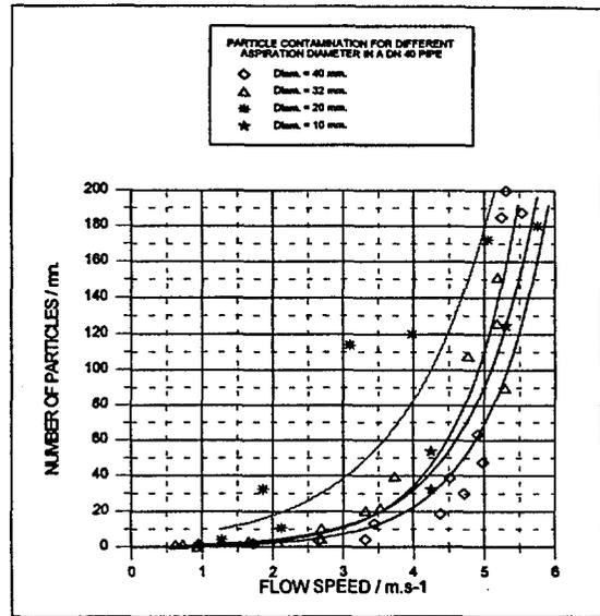
Figure 6.3 : Number of the detected particle ( $0.19\mu\text{m} < \text{size} < 0.5\mu\text{m}$ ) as a function of the flow speed.
