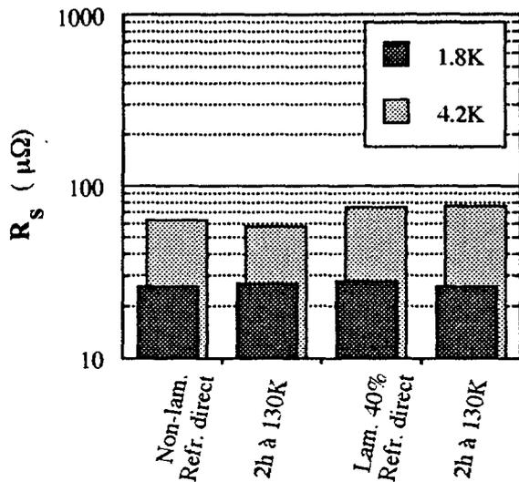
Figure 10. Effect of cold-work on  $R_s$  for RRR = 30 plates. The plates were tested at 5 mm thickness, then rolled to 3 mm thickness and tested again. The plates were chemically polished before each series of tests.
