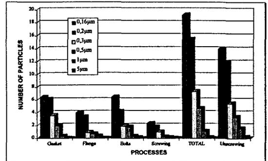
Diagram 2 : Setting of the CF35 flanges Average on 10 gaskets - Pipe of 500 mm. long.
