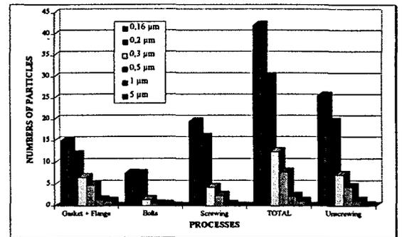
Diagram 3 : Setting of the flanges with an Helicoflex gasket (n°:15040) - Average on 8 gaskets - Pipe of 365 mm. long
