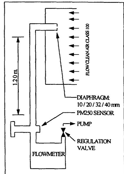
Figure 6.1 : Experimental set-up to measure the particle contamination induced by the flow speed.
