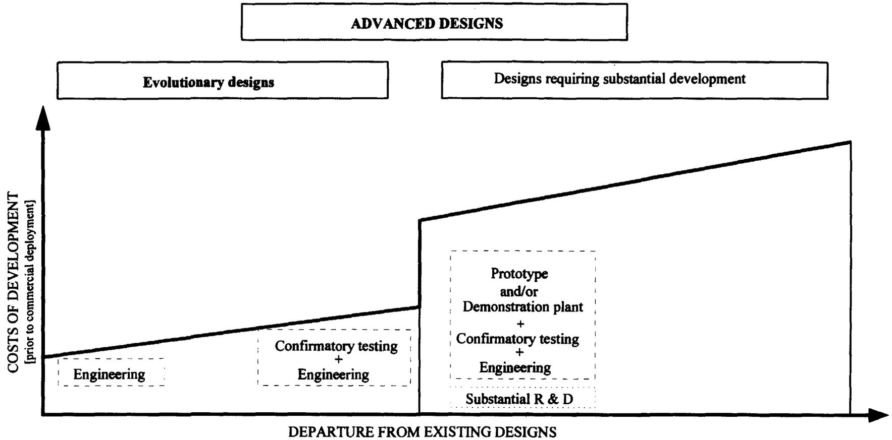
[A prototype is normally a scaled down unit, whereas a demonstration plant is a more substantial plant that can be as large as full size.]
