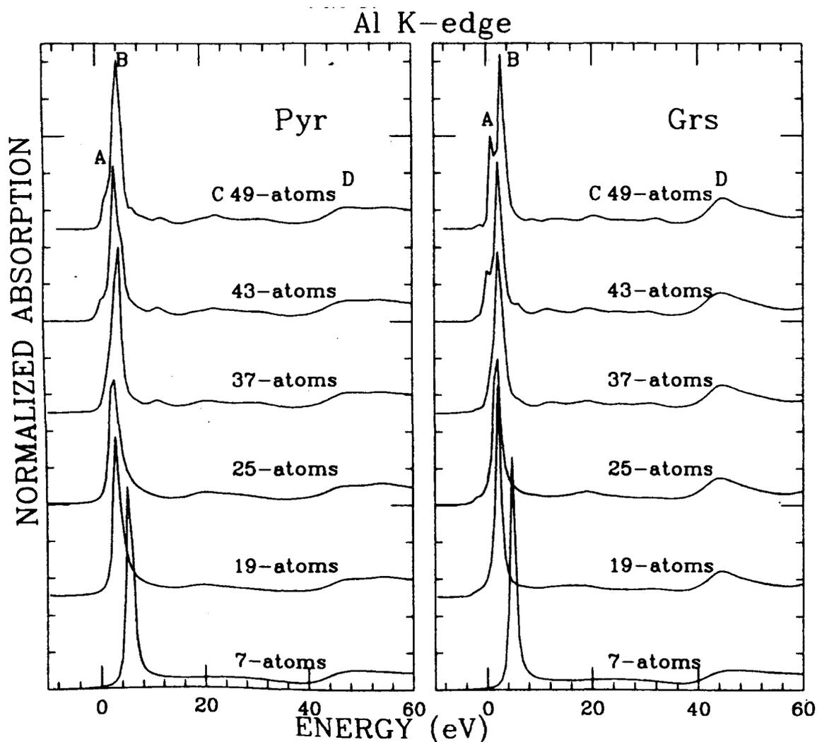
Fig. 2. Theoretical XANES spectra at the Al K-edge as function of the cluster size for pyrope (left panel) and grossular (right panel).
