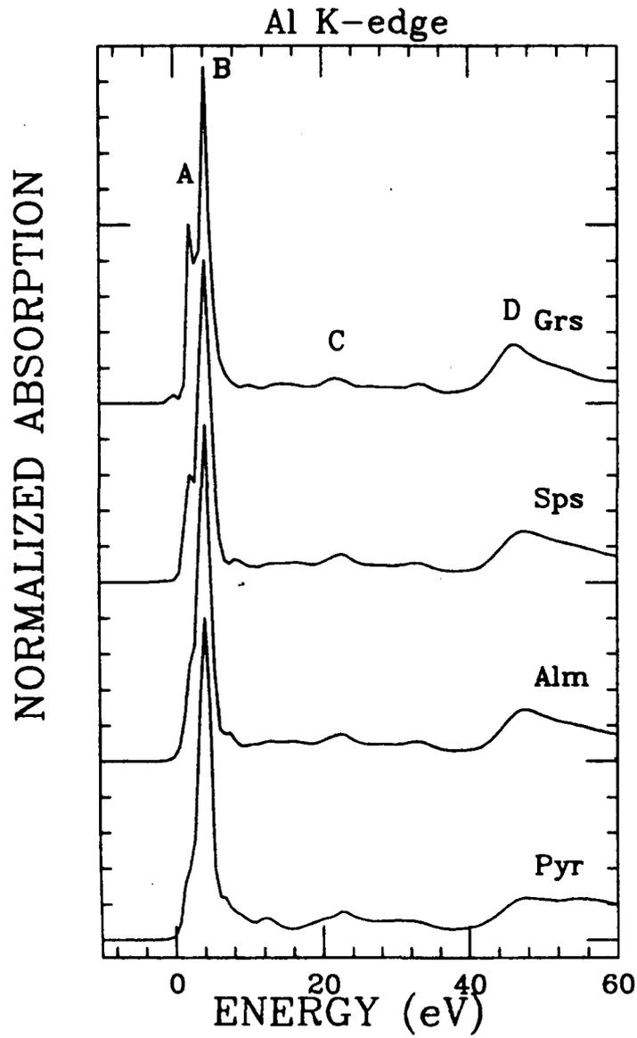
**Fig. 3.** MS calculations of the Al K-edge XANES of the four garnets reported in Figure 1, obtained with clusters of the same size.
