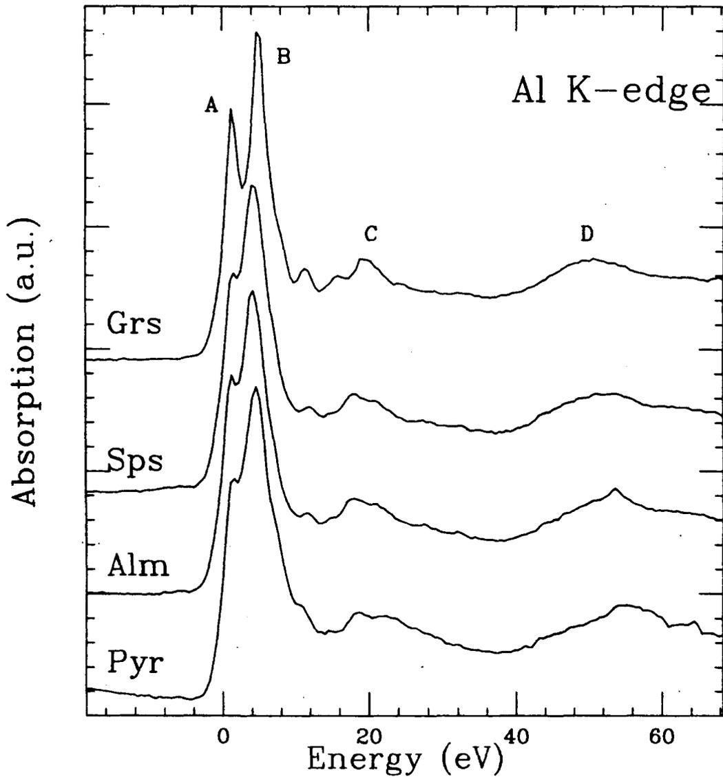
Fig. 1. Experimental Al K-edge XANES spectra for pyrope (Pyr,  $Mg_3Al_2Si_3O_{12}$ ), almandine (Alm,  $Fe_3Al_2Si_3O_{12}$ ), spessartine (Sps,  $Mn_3Al_2Si_3O_{12}$ ) and grossular (Grs,  $Ca_3Al_2Si_3O_{12}$ ).
