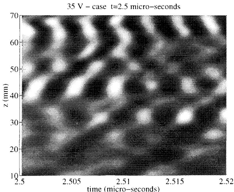
Figure 6: The electric field strength in the simulation of the 35 V case as a function of time and space displayed in a grey-scale plot. The time  $t$  is between 2.50 and 2.515  $\mu\text{s}$ .
