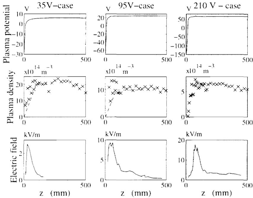
Figure 3: Plasma potential, plasma density and the maximum electric field strength as functions of the axial coordinate  $z$ , for the 35, 95, and 210 V cases. The dashed lines in the experimental density plots of the 35 and 95 V cases show the initial density of the corresponding simulations.
