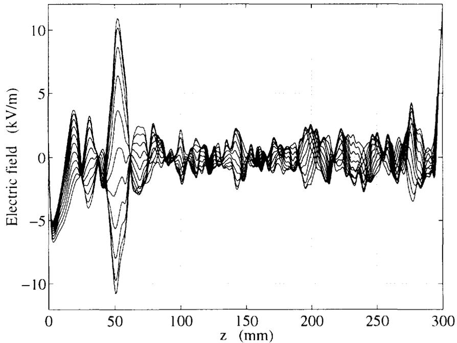
Figure 10: The electric field in the simulation of the 95 volt case for different times  $t$  between  $t = 2.0060 \mu\text{s}$  and  $t = 2.0084 \mu\text{s}$ , with  $\delta t = 0.2 \text{ ns}$  between the curves. The dominating amplitude of the HF spike is more evident than in the grey scale plot of Fig. 8.
