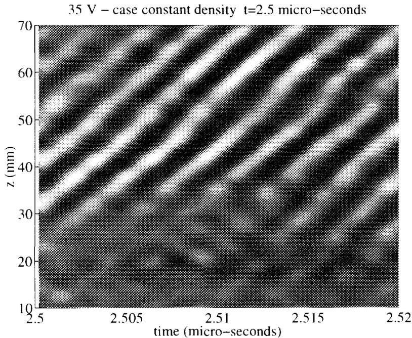
Figure 7: The electric field strength at time  $t$  between 2.50 and 2.515  $\mu\text{s}$  in a simulation where the density is constant, and equal to  $2 \cdot 10^{15} \text{ m}^{-3}$  throughout the simulated system. The other parameters are the same as in the simulation shown in Fig. 6. When the density is constant no HF spike is seen. The dominating wave is forward travelling.
