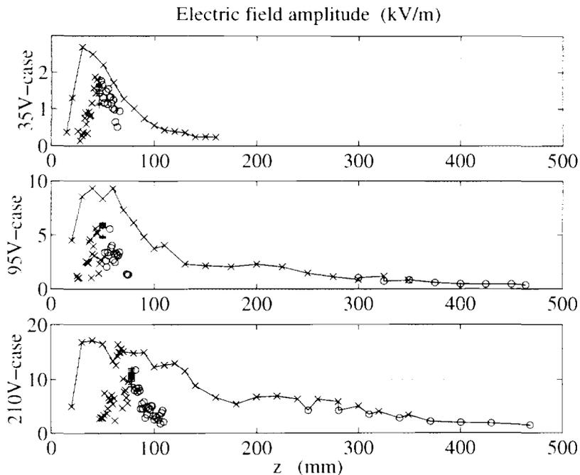
Figure 5: The maximum electric field as a function of  $z$  measured within the same short time interval as is shown in Fig. 4. Measurements made with probe A, which is closest to the cathode, are marked “x”, probe B “+”, and probe C “o”. There is clearly an HF spike, as in the double layer case. The solid curves show the maximum electric field that could be observed as a function of  $z$ .
