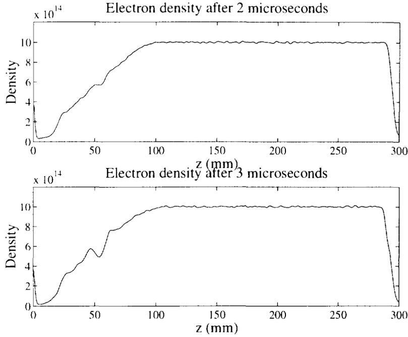
Figure 9: The plasma density after 2 and  $3\mu\text{s}$  respectively. A density dip is observed at the position of the spike.
