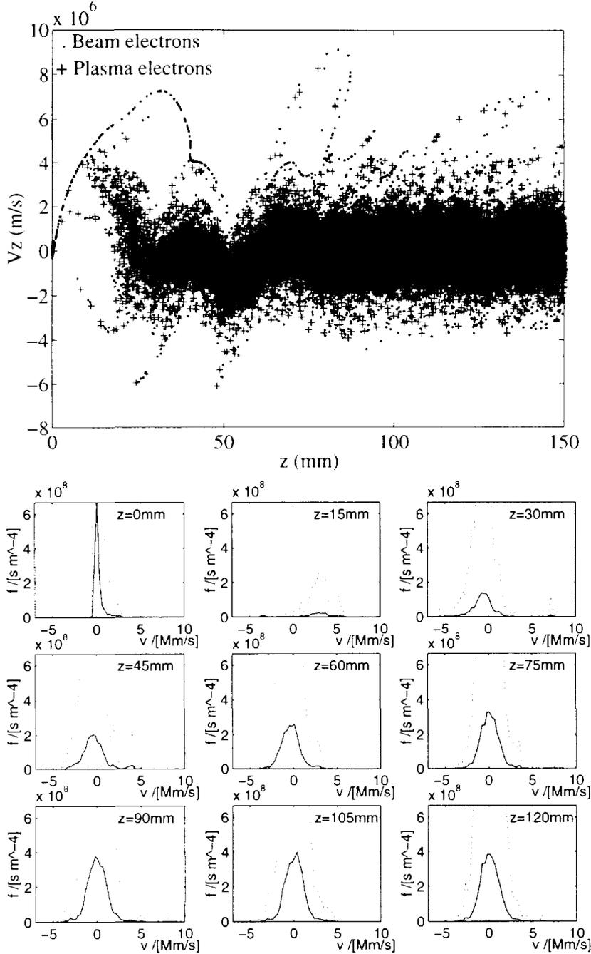
Figure 11: (a) A phase space diagram of the simulated 95 V case at  $t = 2.0072 \mu\text{s}$ . The beam is spread completely after passing the HF spike, at  $z \approx 45\text{mm}$ . To the left of the spike three structures of accelerated particles with negative velocity are evident.
