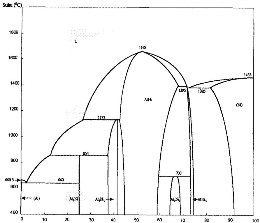
Figure 1. Binary phase diagram for Al-Ni system.
