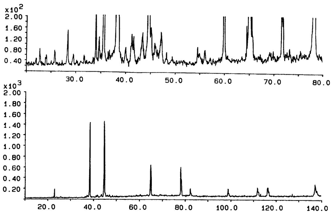
Figure 7. XRD patterns of the Al-Al<sub>3</sub>Ni eutectic composite reinforced SiC (a) 15wt% SiC (b) the bead formed at the surface.
