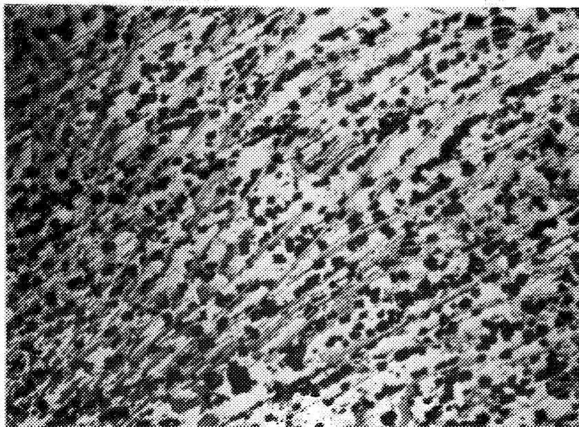
Figure 5. Microstructure of the bead formed at the surface of the composite sintered at 800°C.
