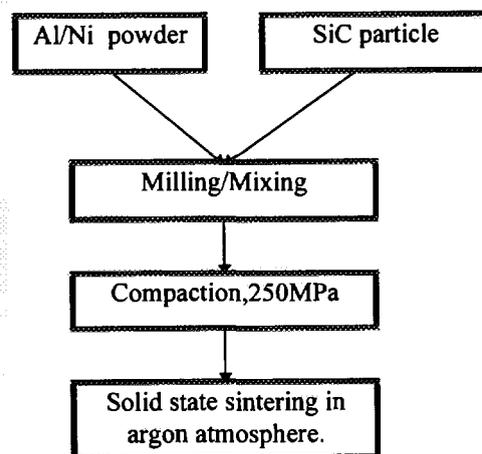
Figure 2. Schematic flow diagram for EPM processing of Al- $Al_3Ni$  eutectic composite reinforced SiC.
