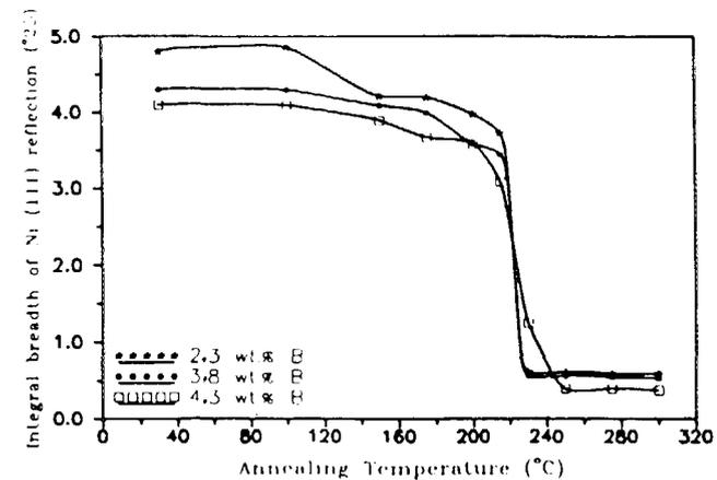
**Fig. 2** Variation of a) ratio of integrated intensities of amorphous and crystalline reflections and b) integral breadth of (111) reflection, with annealing temperature in electroless Ni-B deposits.
