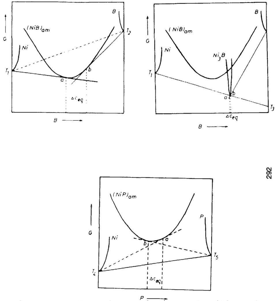
**Fig. 4** Schematic variation of Gibbs' free energy with concentration for a) Ni-B system, prior to the onset of nucleation of  $Ni_3B$  and b) after the nucleation of  $Ni_3B$ . c) prior to the onset of nucleation of  $Ni_3P$  in Ni-P system.
