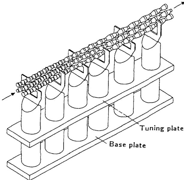
Fig.7 Scheme of a VE-RFQ
