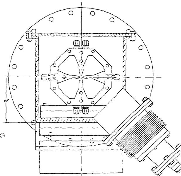
Fig. 5 Cross section of the AccSys PLI/DLI RFQ
