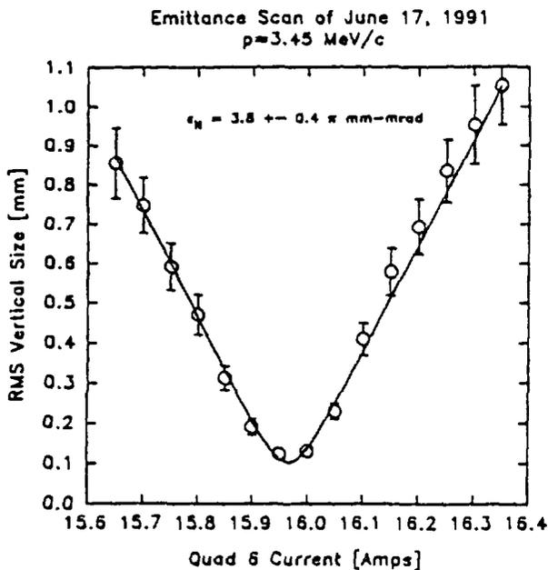
Fig. 4. The vertical projections of the electron beam on a profile monitor as a function of quadrupole current.
