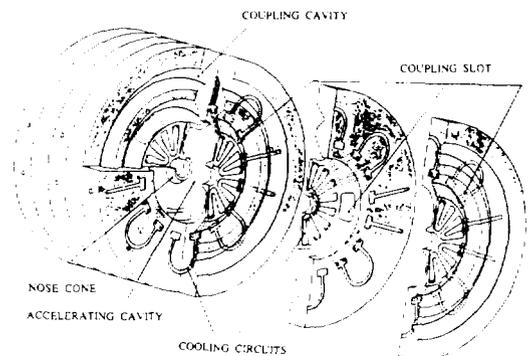
Fig. 1 A Cutaway view of the four-slot ACS of type-S. The slot-orientation is rotated 45 degrees from segment to segment.
