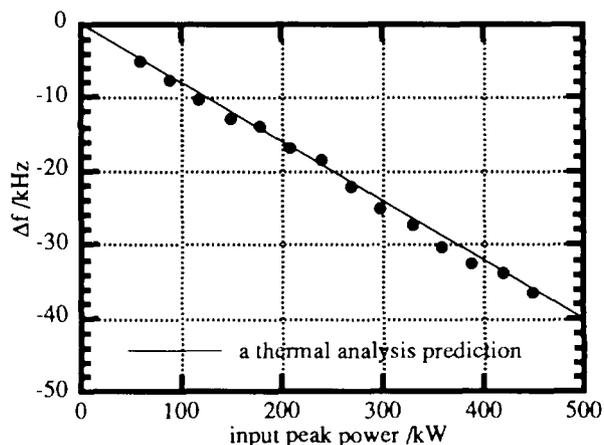
Fig. 4 Measured thermal detuning vs. the input RF peak power.
