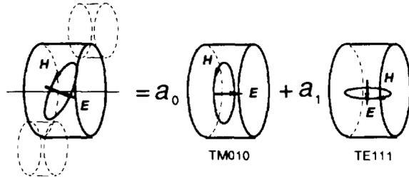
Fig. 6 A schematic drawing showing how the accelerating field is distorted in an SCS cavity.
