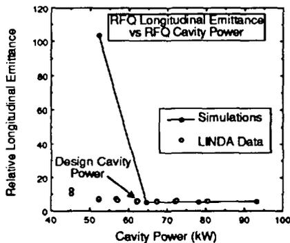
Fig. 7. Relative longitudinal rms emittance vs cavity power.
