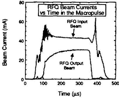
Fig. 2. RFQ input/output beam current versus time.
