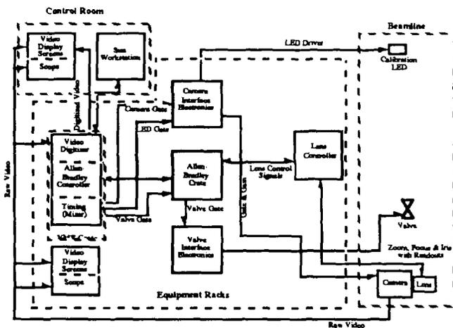
Fig. 2. Video profile diagnostic block diagram.
