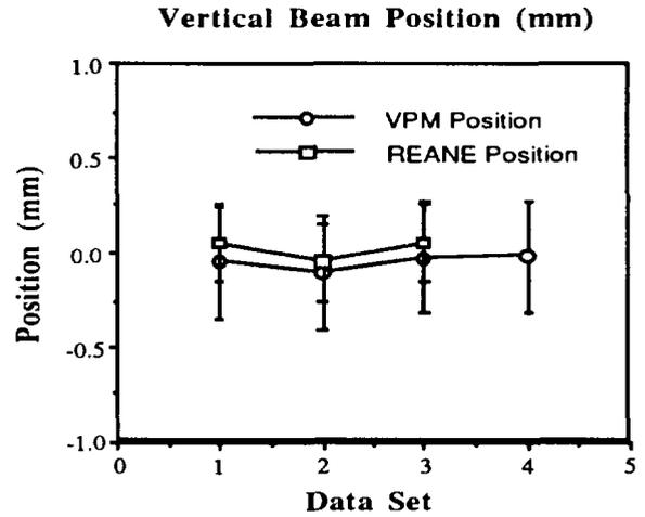
Fig. 6. Vertical beam centroid location as measured using the slit and collector gear and the VPM for several IMS output quad settings.
