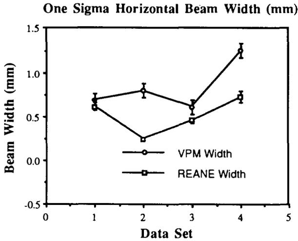
Fig. 4. Horizontal beam widths measured using the slit and collector gear and the VPM for several IMS output quad settings.
