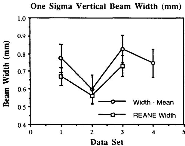
Fig. 5. Vertical beam widths measured using the slit and collector gear and the VPM for several IMS output quad settings.
