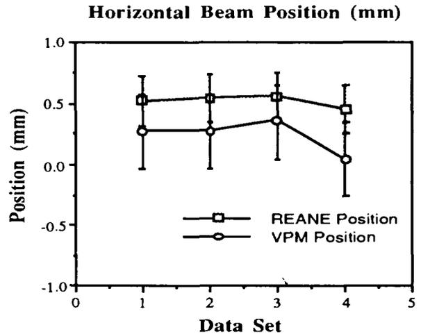
Fig. 7. Horizontal beam centroid location as measured using the slit and collector gear and the VPM for several IMS output quad settings.
