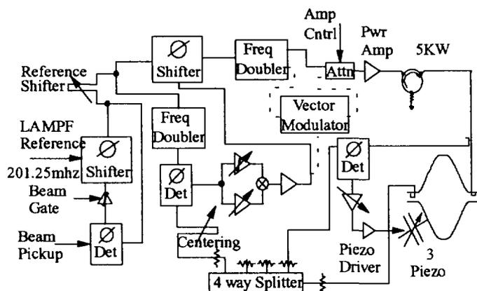
Fig 2. Control with drive from frequency reference.
