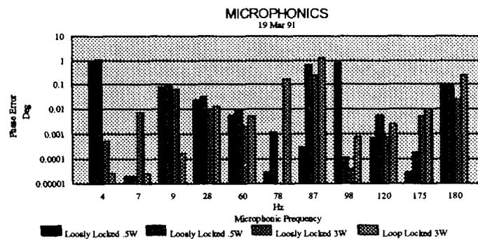
Fig 4. Phase Error due to Microphonic Vibrations.
