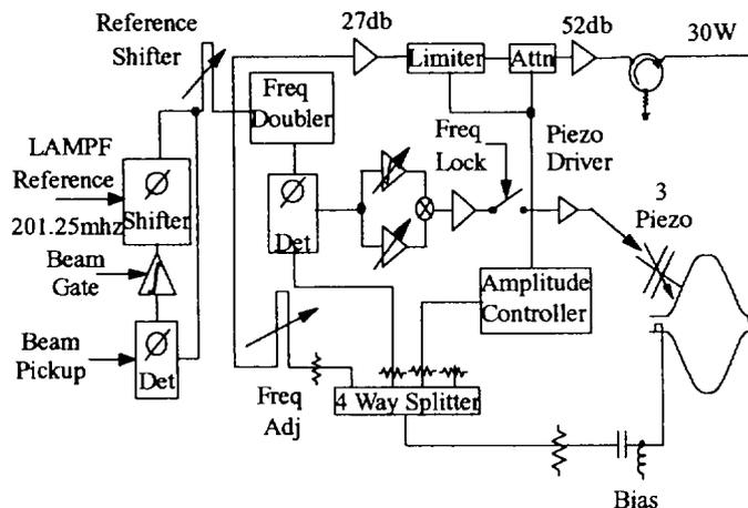
Fig 3. Control for the self oscillating mode.
