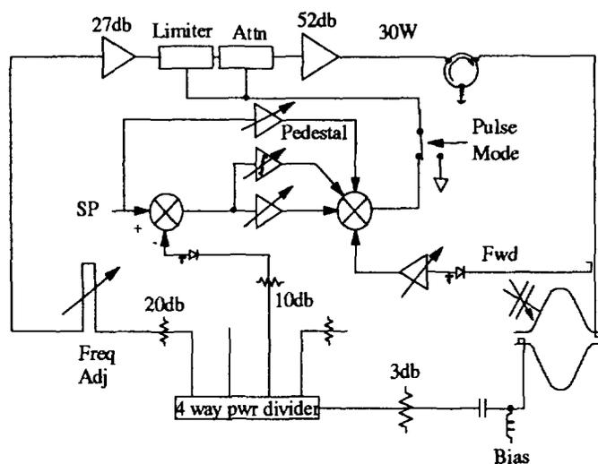
Fig 1. Amplitude Controller for Cell.
