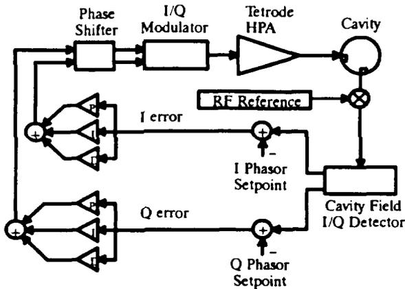
Fig. 3 Functional block diagram of cavity field control system.
