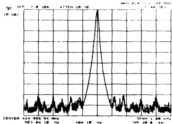
Fig. 2 RF reference spectrum input to feedback loop.
