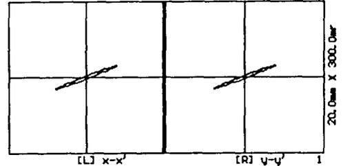
Fig. 2 beam ellipse of high current mode in phase space.
