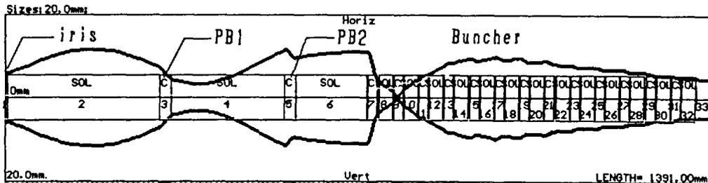
Fig. 4 beam envelope of high current mode.
