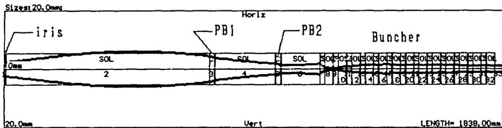
Fig. 3 beam envelope of low current mode.
