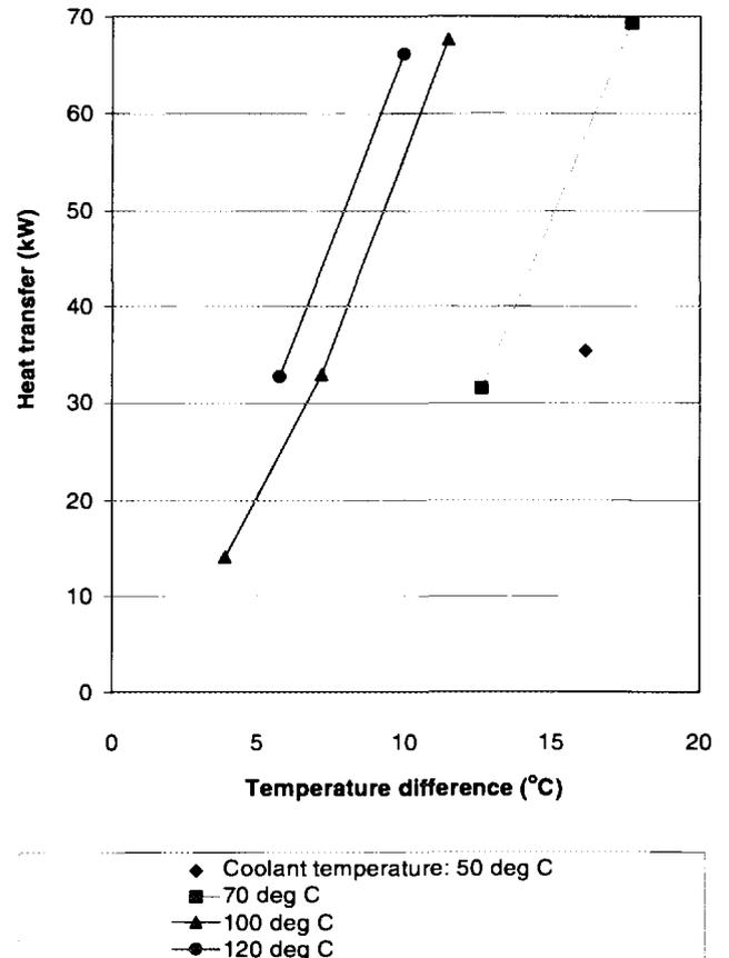
**Fig. 5:** Effect of coolant temperature on heat exchanger performance at constant gas flow rate (0.3 kg/s) and air partial density (1 kg/m<sup>3</sup>).
