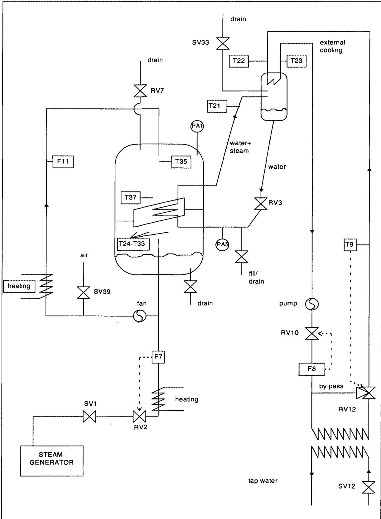
**Fig. 2:** LINX-2 configuration for ENEL internal heat exchanger tests.
