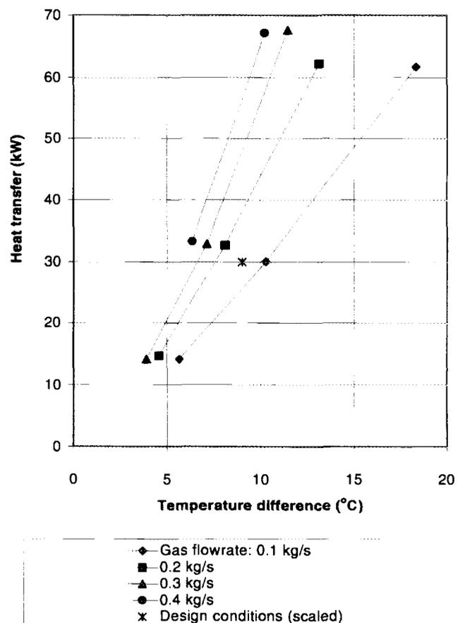
**Fig. 3:** Effect of gas flow rate on heat exchanger performance at constant air partial density ( $1 \text{ kg/m}^3$ ) and coolant temperature ( $100^{\circ}\text{C}$ ).
