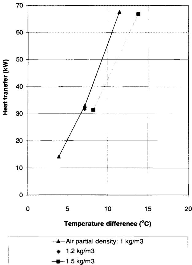
**Fig. 4:** Effect of air partial density on heat exchanger performance at constant gas flow rate (0.3 kg/s) and coolant temperature (100°C).
