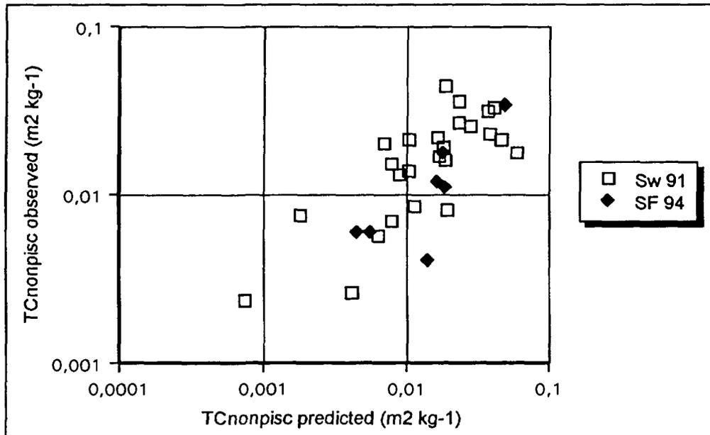
Figure 4. Observed and predicted transfer coefficients of  $^{137}\text{Cs}$  from Chernobyl fallout to non-piscivore fish in 41 Swedish lakes during 1991 and in lakes of 7 regions in Finland during 1994.
