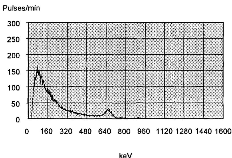
Figure 3. Example of an *in situ* gamma spectrum, indicating the  $^{137}\text{Cs}$  deposition at Tangen farm 10.09.96 with a peak at 661 keV.
