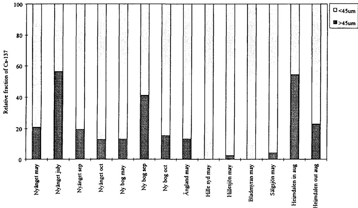
Figure 6. Composition of particulate Cs-137 in water at different times of the year.
