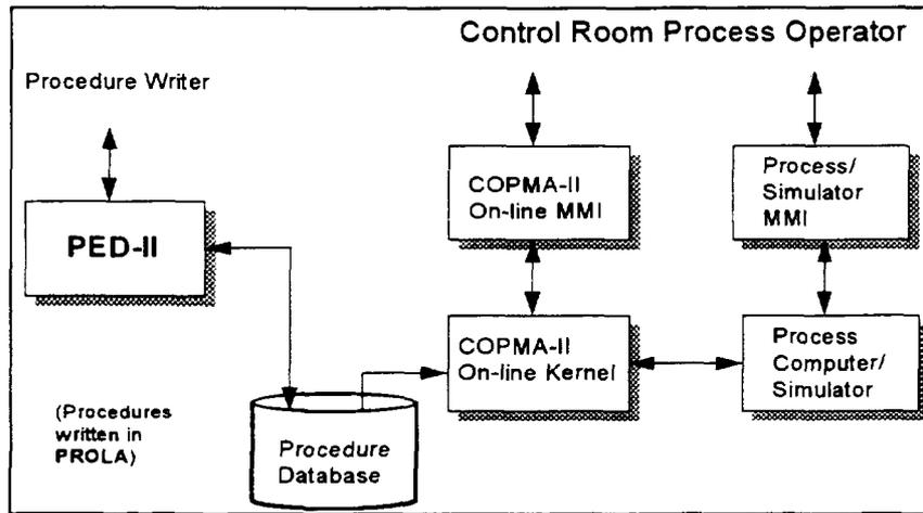
FIG. 4. COPMA-II system components.
