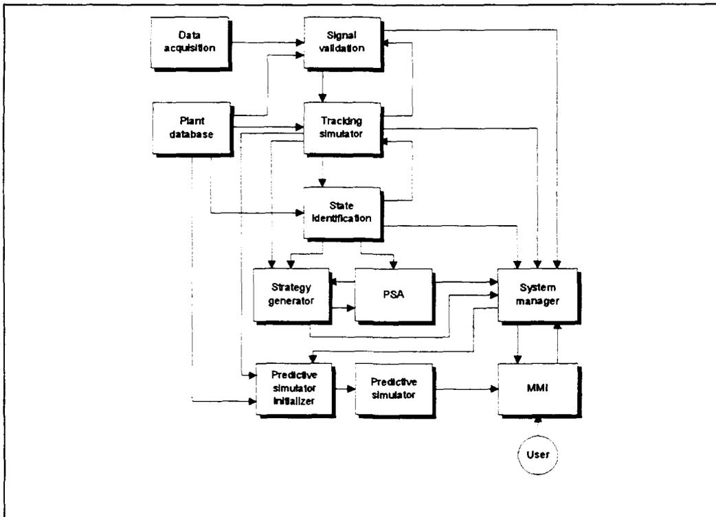
FIG. 5. Block diagram of the CAMS system.
