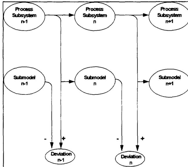
FIG. 2. The principle of model-based early fault detection.
