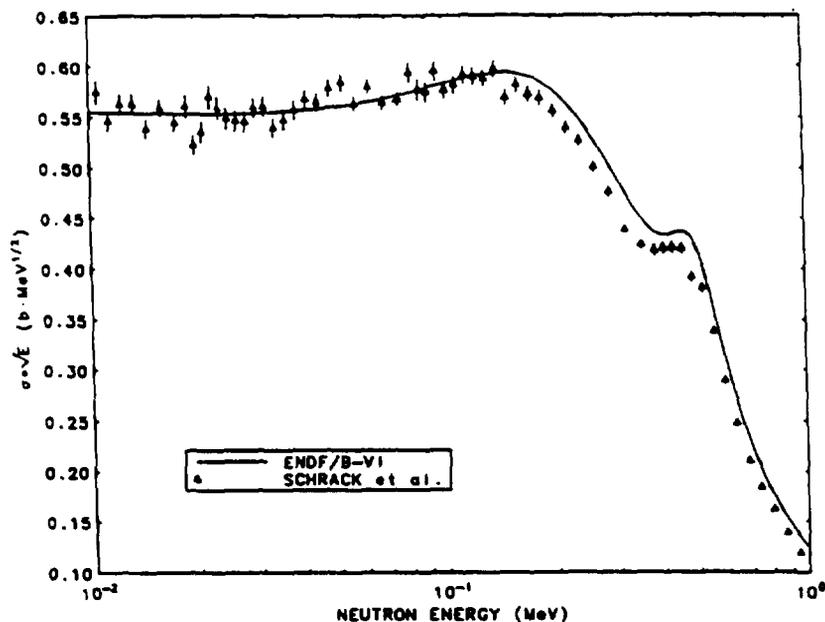
Fig. 3 Measurements of the  $^{10}\text{B}(n, \alpha, \gamma)$  cross section by Schrack *et al.* [6] compared with the ENDF/B-VI evaluation.
