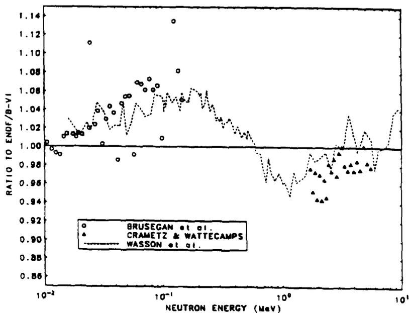
Fig. 4 Comparison of the recent measurements of the  $^{10}\text{B}$  total cross section by Brusegan *et al.* [7], Crametz and Wattecamps [8], and Wasson *et al.* [9] with the ENDF/B-VI evaluation.
