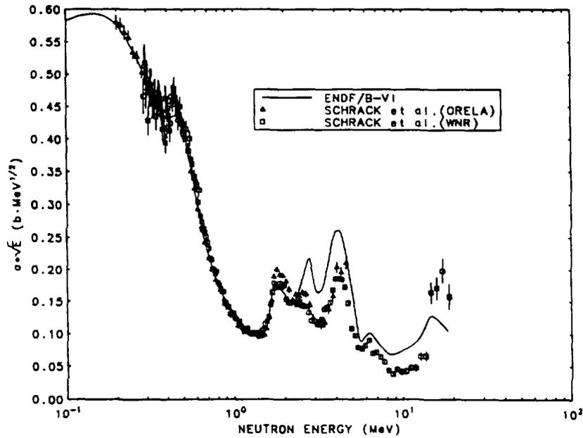
Fig. 2 Comparison of the  $^{10}\text{B}(n, \alpha, \gamma)$  cross section measurements of Schrack *et al.*, at ORELA [4] and WNR [5] facilities with the ENDF/B-VI evaluation.
