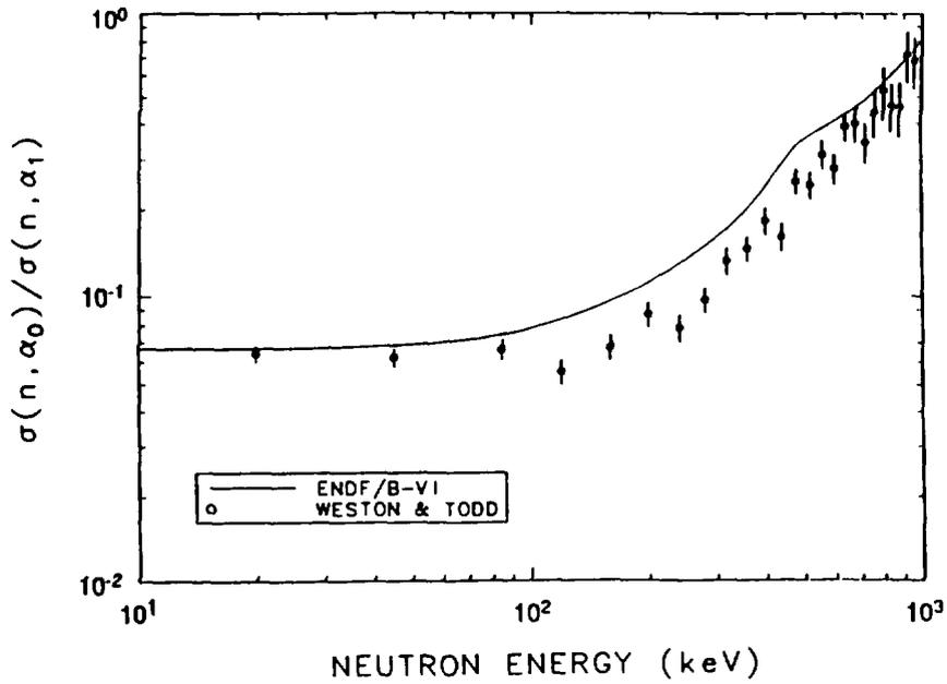
Fig. 1 Measurements of the branching ratio of  $^{10}\text{B}$  cross sections by Weston and Todd [3] compared with the ENDF/B-VI evaluation.
