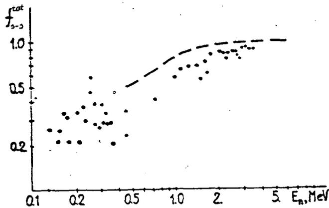
FIG. 4. Self-shielding factors of iron cross-sections from Ref. [15]. The points represent experimental data from measurements for transmission in thick specimens and the broken line the results of calculation from experimental data (point curves of cross-sections), measured with high resolution.
