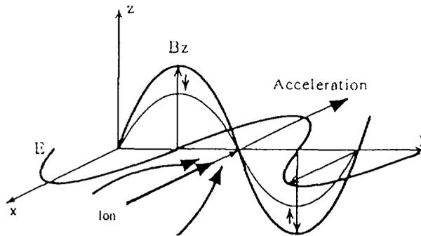
Fig. 1 A static spatially alternating magnetic field  $B_z$  is first generated and is abruptly decoupled from the electric circuit which generates  $B_z$ . During the demagnetization phase a high acceleration field  $E$  is induced. Ions are accelerated by  $E$  and focused by  $B_z$ .
