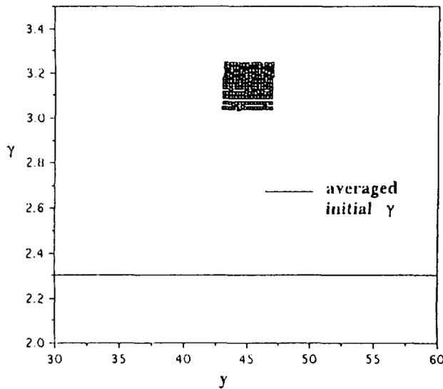
Fig.3 An ion map by particle simulation. The ion relativistic factor  $\gamma$  versus  $y$  at the maximum acceleration time. The initial ion speed is  $0.9c$  on average, the beam initial temperature is  $10\text{ eV}$ , and the maximum  $\gamma=3.24$ . The ions are accelerated well.
