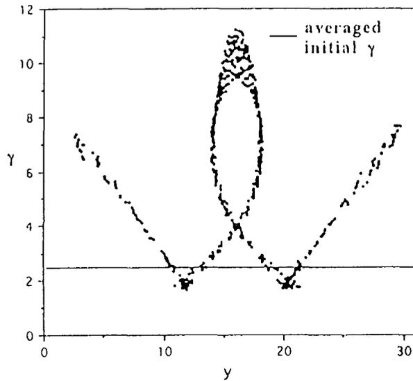
Fig. 2 A particle map by particle (PIC) simulation. The electron relativistic factor  $\gamma$  versus  $y$  at the maximum acceleration time. The initial electron speed is  $0.9c$  on average, the beam initial temperature is  $10\text{ eV}$ , and the maximum  $\gamma=11.5$ . A fraction of the electrons is accelerated well.
