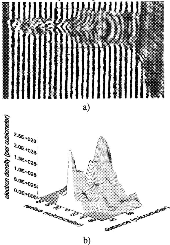
Fig.2. The interferogram (a) and electron density distribution (b) for delay time  $t=1.16$  ns after ignition.
