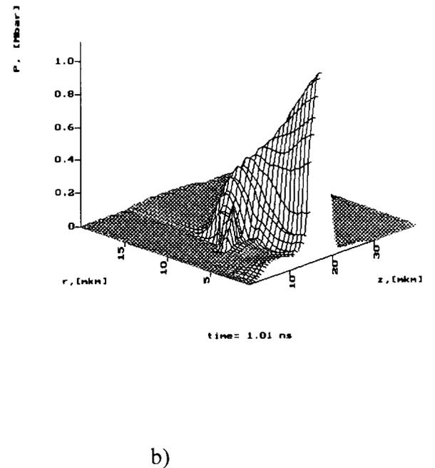
Fig.3: The distributions of density (a) and pressure (b) of matter at  $t=1.0$  ns.
