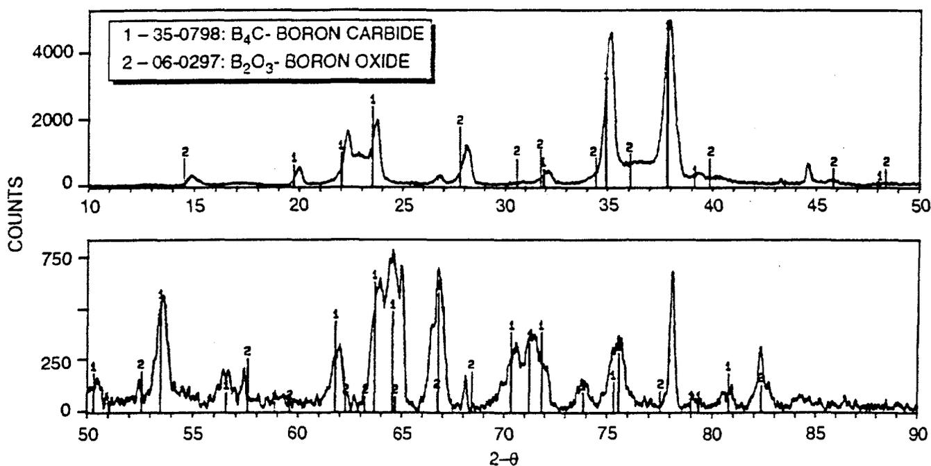
Fig. 2. XRD pattern for plasma-spray-deposited  $B_4C$ .
