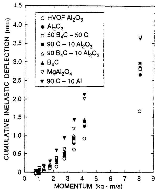
Fig. 8. Cumulative inelastic deflection vs momentum for low-velocity impact of steel spheres.
