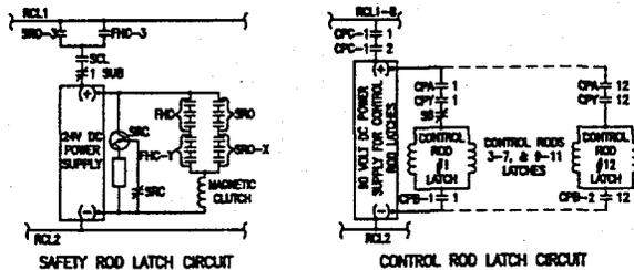
Figure 3. Control and Safety Rod Latch Circuit.
