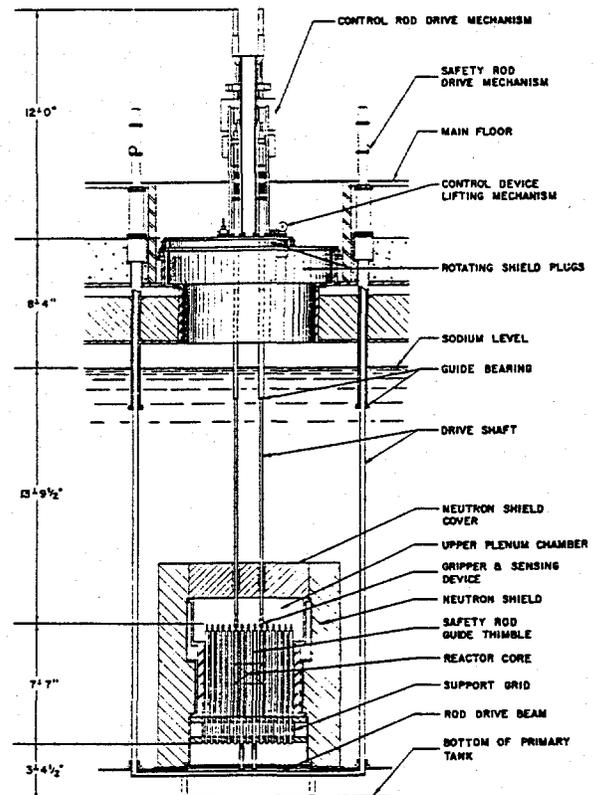
Figure 2. Control and Safety Rod Drive System.
