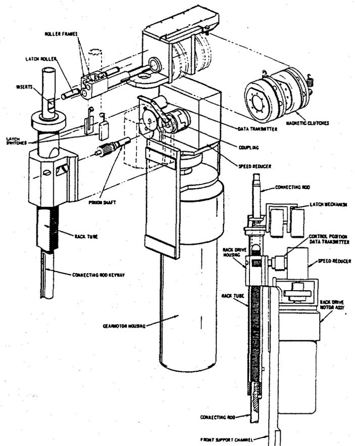
Figure 1. Control Rod Drive Shaft Mechanism.
