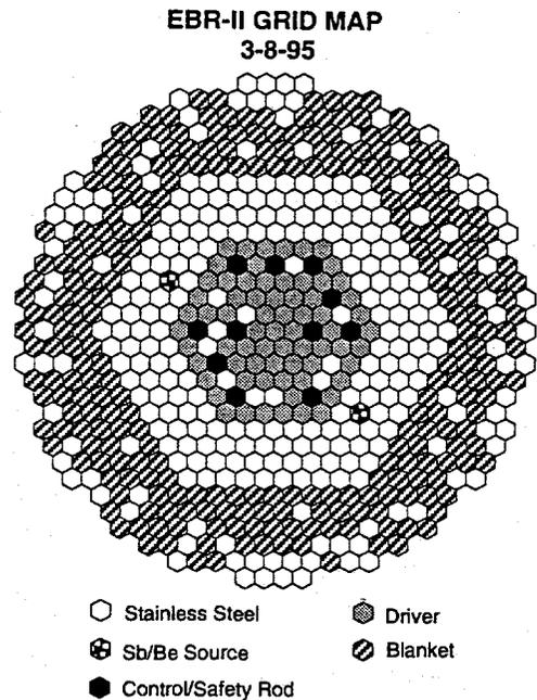
Figure 4. EBR-II Grid Map for RDF-1 Loading.
