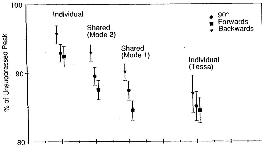
Figure 5 Comparison between suppressed and unsuppressed spectra to determine loss rates due to suppression. The terms are defined in the text. The forward angle used was 72°, the backward angle used was 158°.
