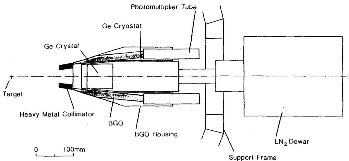
Figure 1 The escape suppressed spectrometer to be use in the first phase of EUROGAM.
