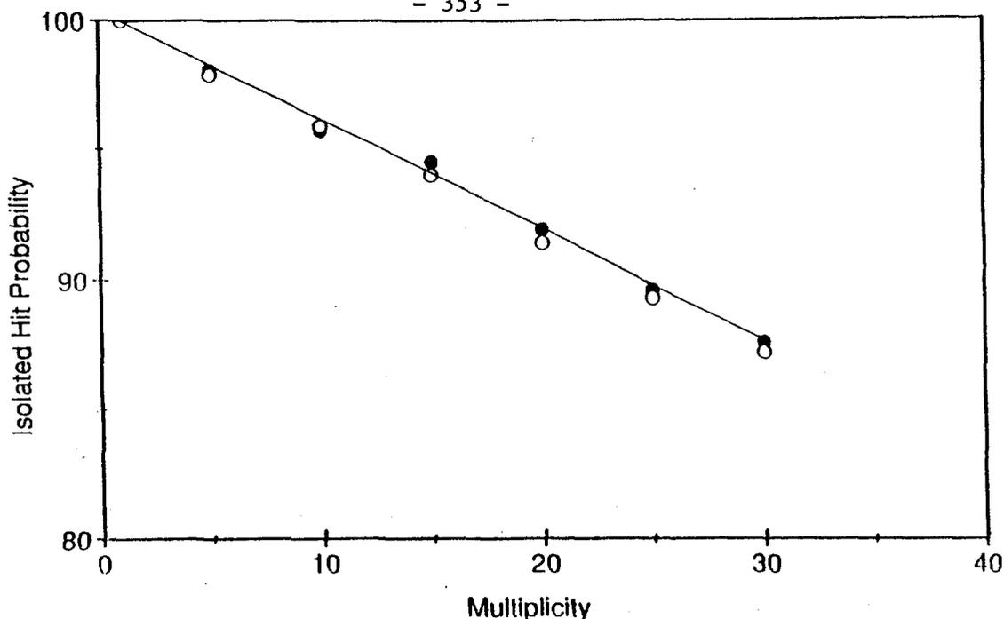
Figure 7 Isolated hit probability measured (see text) as a function of gamma ray multiplicity for  $^{60}\text{Co}$  (1.33MeV) and  $^{207}\text{Bi}$  (0.57MeV).
