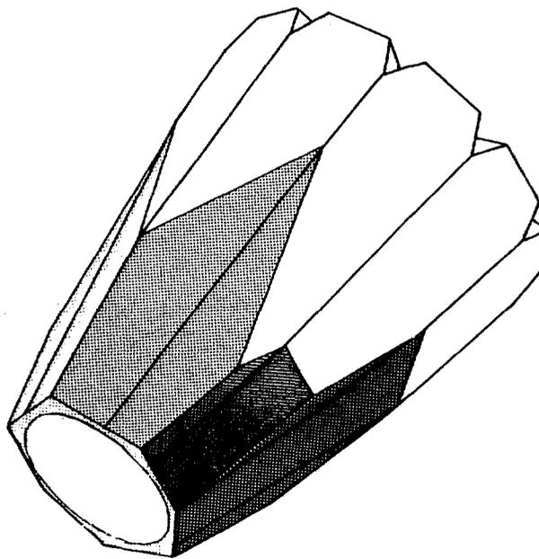
Figure 2 Schematic drawing of the BGO shield to be used in EUGOGAM. It consists of 10 optically isolated elements.
